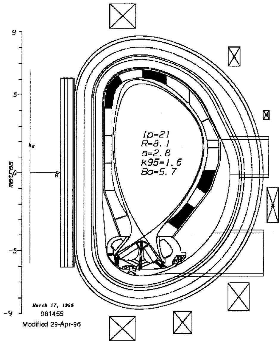
Figure 2: Cross Section elevation of ITER. Shaded regions show suggested locations of activation irradiation ends.
