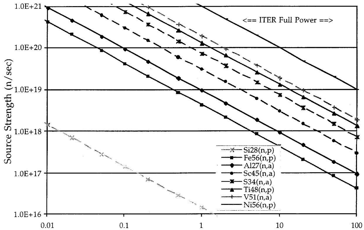
Figure 1: Source strength required to create 100 microCuries of activity in a 100 second exposure for a given mass of material. Irradiation location at top of machine (foil radius 8.7 m, foil height 6.0 m, poloidal angle 85°). Reactions are listed from most sensitive to least.
