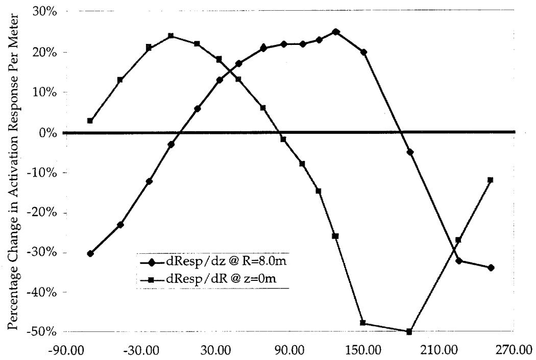
Figure 3: Percentage change in activation response per meter as toroidal line source of neutron emission is moved. The diamonds are caused by variation in the  $z$  direction, and the squares are for variation in the  $R$  direction. Zero degrees is the outboard midplane.
