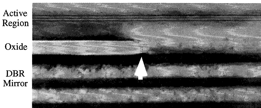
Fig. 5. Cross section TEM image ( g=(311) ) of a VCSEL with an \text{Al}_{0.98}\text{Ga}_{0.02}\text{As} oxide layer; the arrow denotes the oxide terminus.
