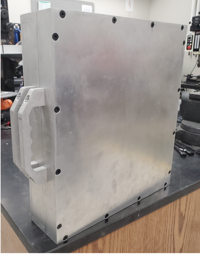
Fig. 1: The front of the full-panel neutron radiography system designed around the ROSSPAD module.
