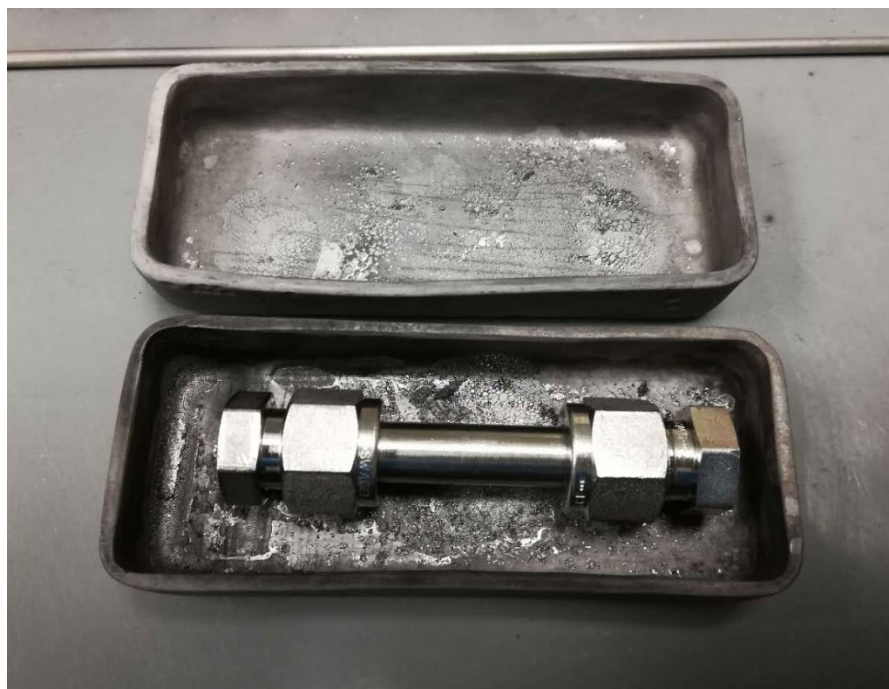
Figure S2. Stainless steel tube for MR reaction.
