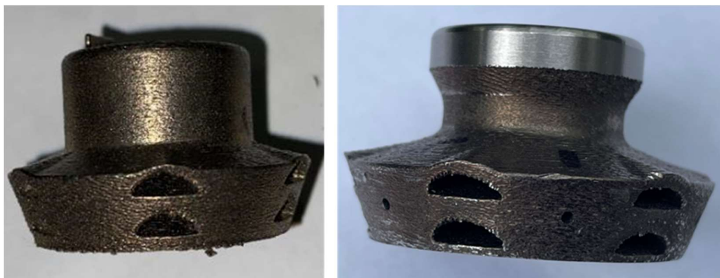
Figure 16: Images of a CS insert after printing (left) and after finish machining (right).
