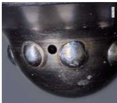
Figure 6: Image of fuel injector used in optical engine
