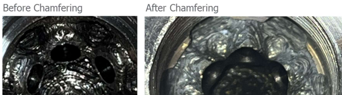
Figure 39: Image of fuel passage inlets before chamfering and after chamfering.
