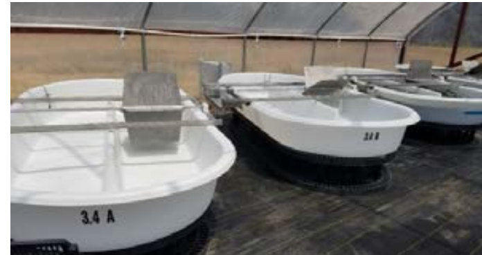
Top: 1-acre ponds at QH, used to measure ingassing rates at a commercially relevant scale. Bottom: MBE 3.4 m 2 used to more fully parameterize air-CO 2 flux.
