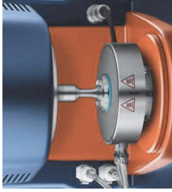
Measured on a Pelletier plates DHR Rheometer
