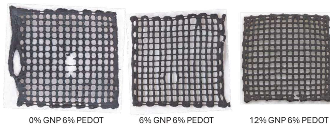
Figure 3: Optical microscope images of printed polymer lattice electrodes, with the ink concentration of PEDOT:PSS and GNP under each.
