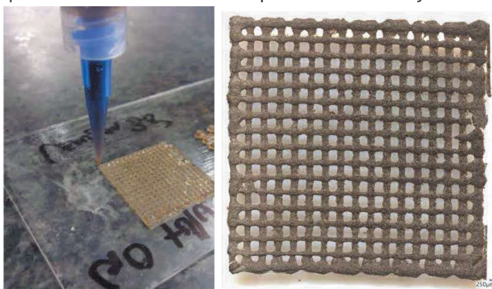
Figure 7: GO Emulsion ink during printing and after freeze drying
