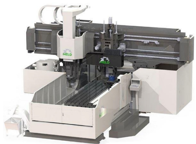
Fig. 12. MELD Manufacturing Corporation 3PO hybrid machine tool with additive head (left) and subtractive head (right) [136].
