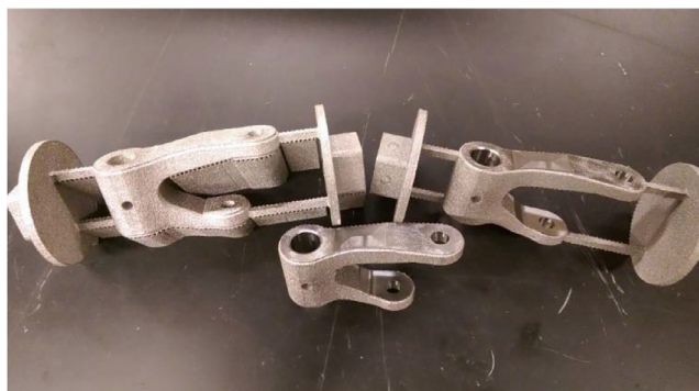
Fig. 66. Powder bed preforms including fixturing features for machining [64].
