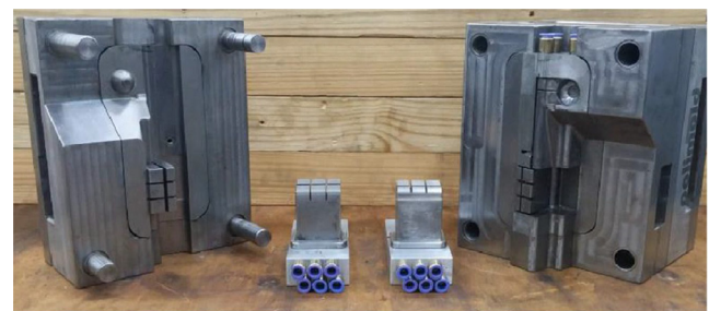
Fig. 46. Mold cavities and the exchangeable inserts (baffle and conformal cooling) [133].
