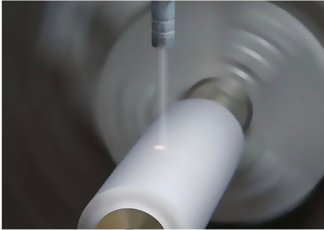
Fig. 14. Hermle cold spray coating deposition, from [78], courtesy HERMLE AG.
