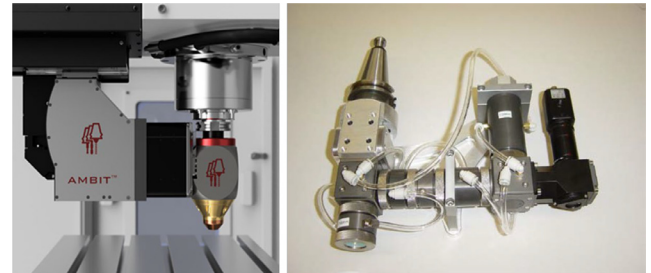
Fig. 27. Retrofit spindle mounted deposition heads showing auxiliary connections [82,146].
