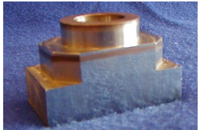
Fig. 55. Copper clad on a nickel-based alloy, Reproduced from [102], with the permission of the Laser Institute of America.
