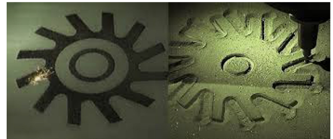
Fig. 17. Matsuura laser powder bed hybrid machine tool work zone during additive (left) and subtractive (right) processes [134].
