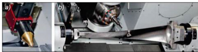
Fig. 52. Hybrid additive/subtractive repair of the edge of a large turbine blade [70].
