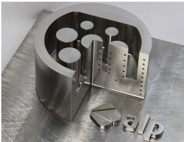
Fig. 73. Hybrid injection mold with conformal cooling. The example is for a charge socket for an electric vehicle [182].
