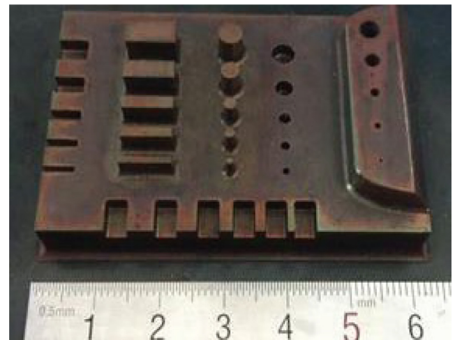
Fig. 18. AISI 18Ni (300) maraging steel part produced using a Sodick OPM Series hybrid machine tool [49].
