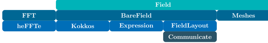
Figure 3: Design layout of fields in IPPL. The underlying data structure is a Kokkos View. IPPL provides an interface to the Fourier transform routines of heFFTe.
