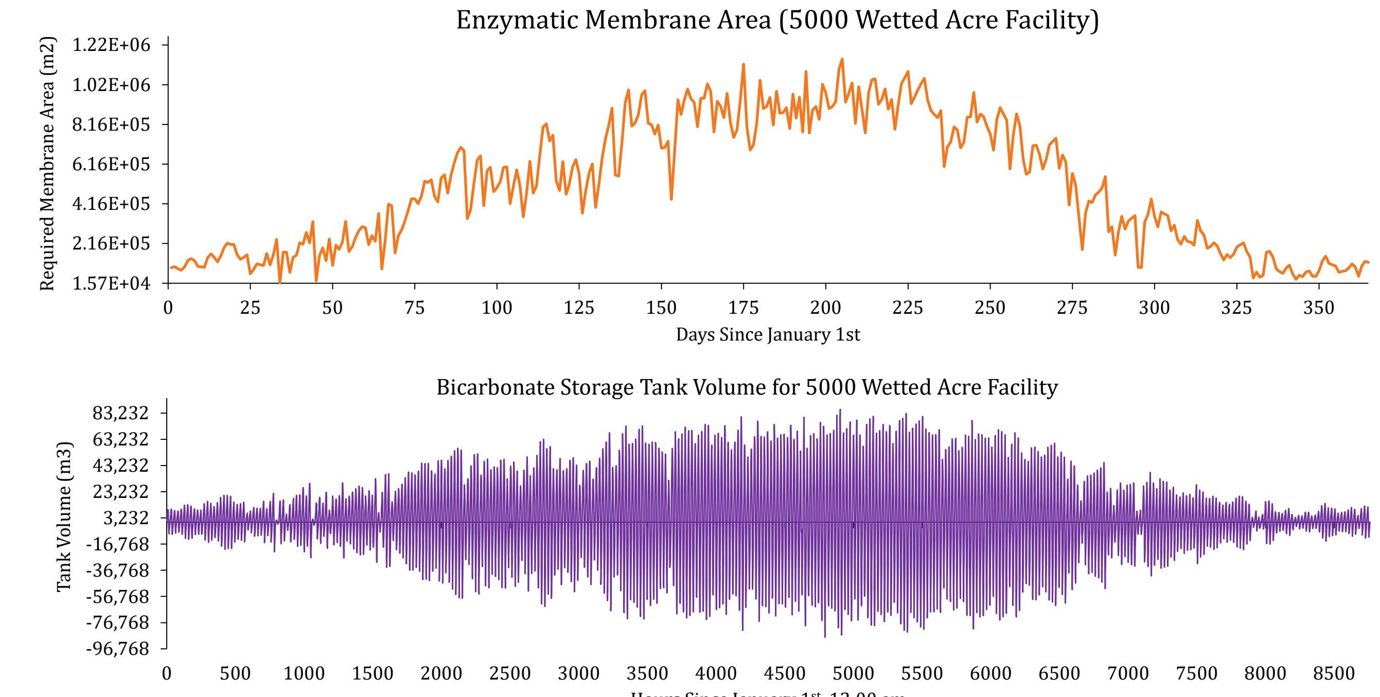
Detailed mass transfer modeling was used in conjunction with hourly growth projections to determine time-resolved inorganic carbon (iC) demands across the facility. Experimentally determined membrane carbon fluxes (moles iC m<sup>-2</sup> s<sup>-1</sup>) and facility-wide flowrates were used to determine the required membrane area as well as the required bicarbonate storage tank volume.
