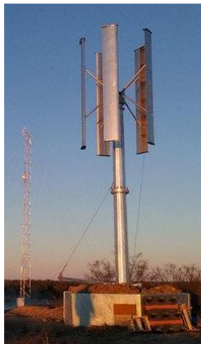
Figure 3: Vertical axis wind turbine (Van Bang Nguyen 2017)
