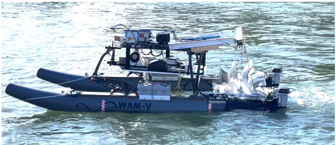
Figure 23: Waterwheel and PTO onboard WAM-V during field testing (Dhanak 2023)
