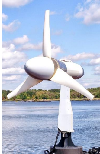
Figure 2: Horizontal axis underwater turbine (Verdant Power n.d.)
