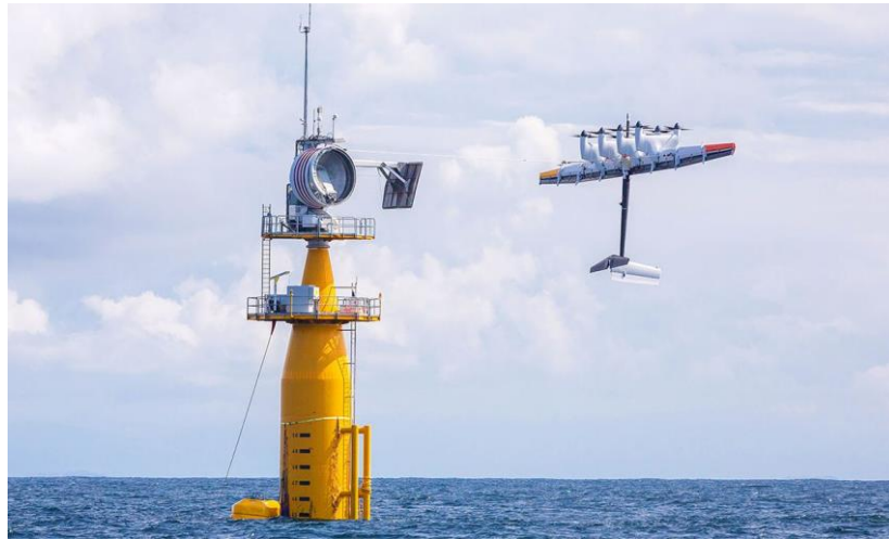
Figure 11: Energy kite under field testing (Anderson 2019)
