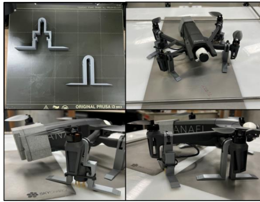
Figure 15: The retrofitted ANAFI Parrot, with costume landing gear
