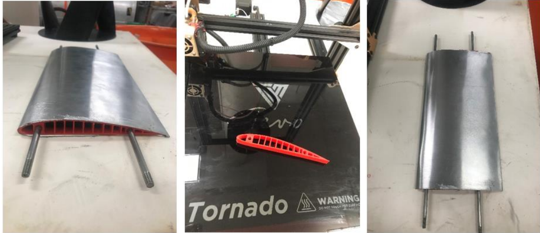
Figure 9: Concentrator prototype (left/right) and 3D printed support section (middle)
