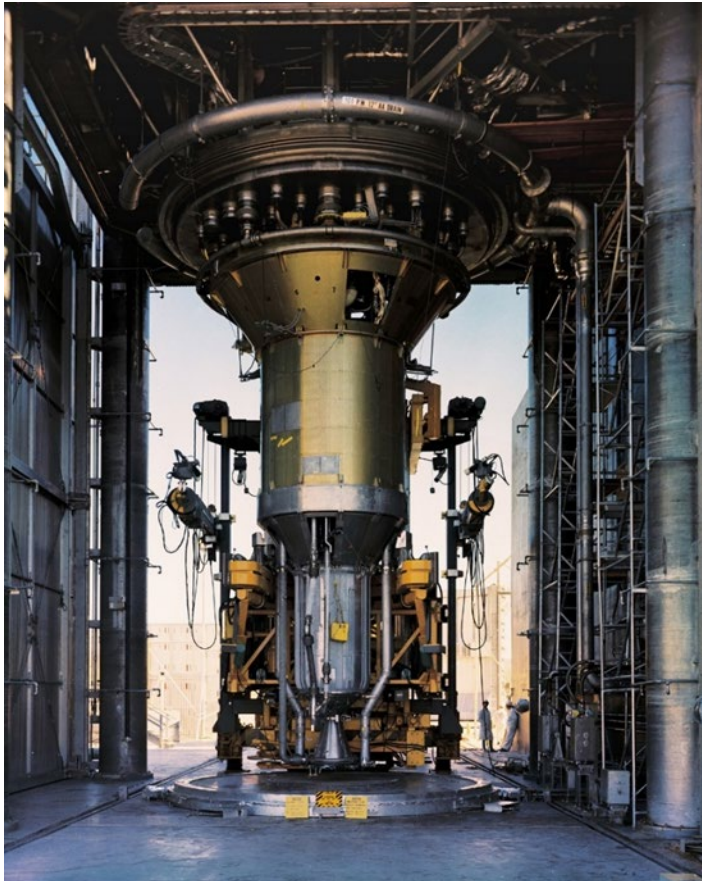
Figure 127. Installation of the XE Prime engine at ETS-1 (photo RSL 5-00164-D06_2098).
