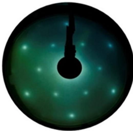
Figure S3: LEED pattern of the intercalated system obtained at E = 100 eV. The LEED pattern indicates a homogenous and well-developed surface. It is the overlapping of the (1 \times 1) graphene spots (outermost) and the (\sqrt{3} \times \sqrt{3}) R30^\circ superstructure spots (inner ones), as expected.
