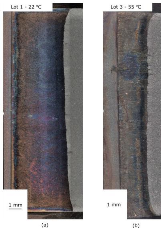
Figure 86: Fractography for samples ran in saturated \text{MgCl}_2 on various lots, temperatures, and directions. The figures correspond to (a) SN0028 (Lot 1 - 22 °C) and (b) SN0095 (Lot 3 - 60 °C). It is noted that if the directions are not noted they are performed in the L-T direction.
