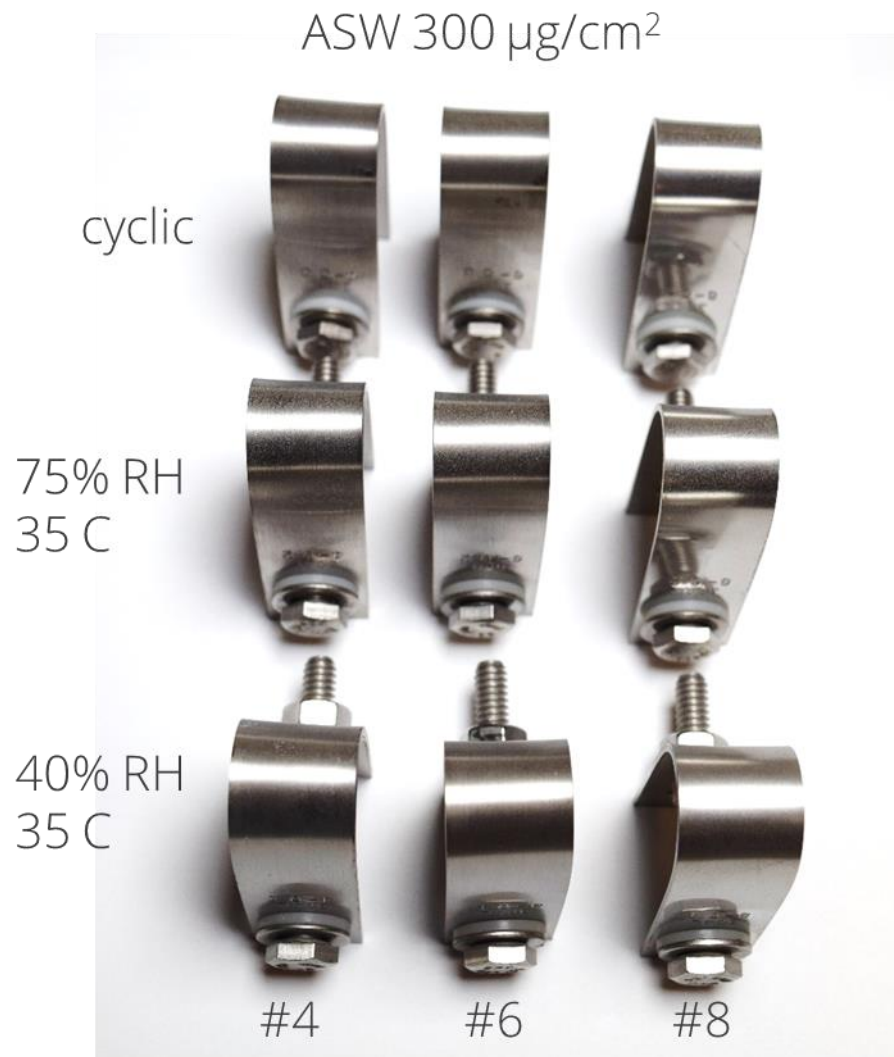
Figure 69. Optical images post 3-day atmospheric exposure of the U-bend samples finished to three different surface finishes.
