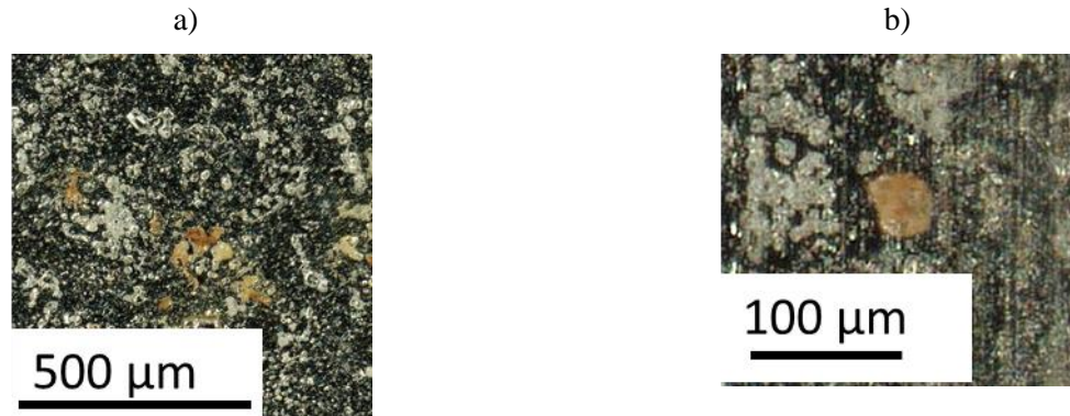
Figure 70. Example higher resolution optical images of post-exposure corrosion damage on a) the #8 surface finish diurnal cyclic exposure and b) the #4 surface finish 75 %RH static exposure.
