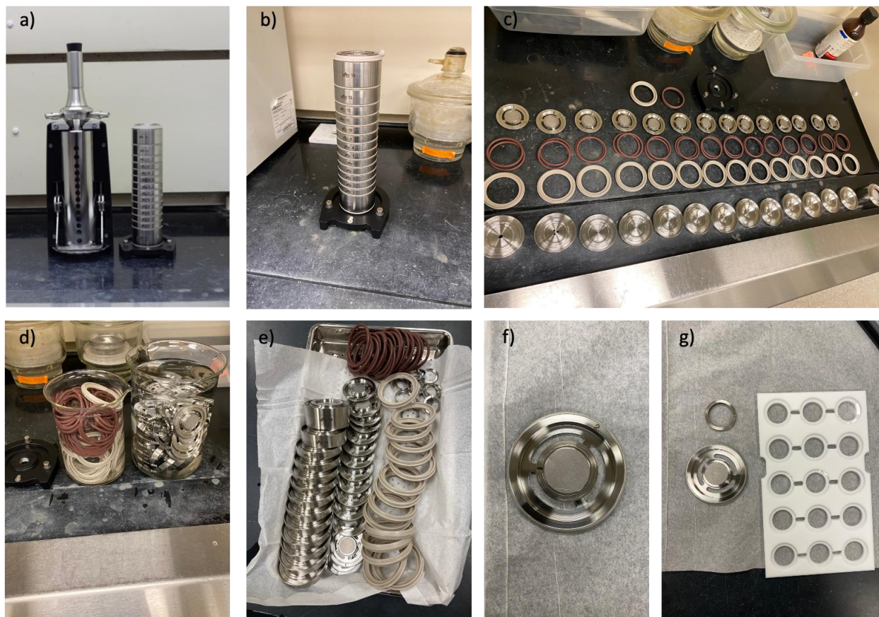
Figure 34. Photos demonstrating the disassembly of the cascade impactor column (a-c), cleaning of each component (d-e), and mounting the greased polycarbonate targets on a impactor stage (f-g).
