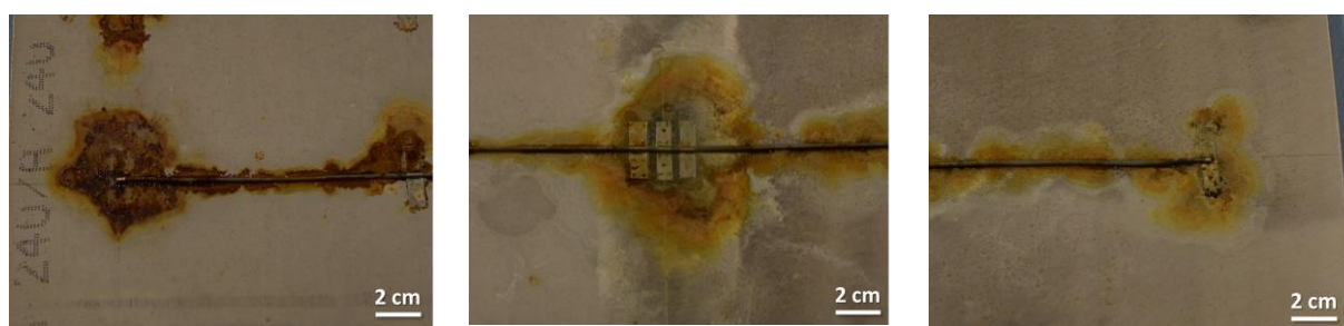
Figure 28. Select shim locations (same as Figure 25) versus exposure time after redeposition of sea salt and second exposure (left on mill scale, center in the weld, and right on ground surface).
