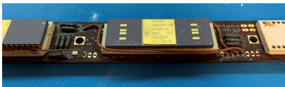
Figure 18. Custom SNL HT application specific integrated circuit (ASIC) programmer for the HT83C51. Utilized for programming the microcontroller while operating at elevated temperatures.
