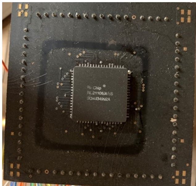
Figure 27. RC2110836 low temperature soldered to Rogers 3003 PCB with HT wires. Pictures of the packaged device were not taken before the oven evaluation. Originally the board was a green color.
