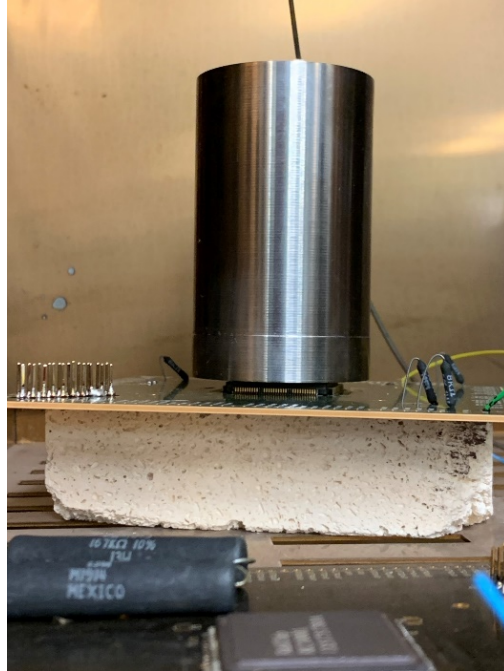
Figure 31. RC10001 microcontroller with a metal weight on top to mitigate deformation under elevated temperature evaluation.
