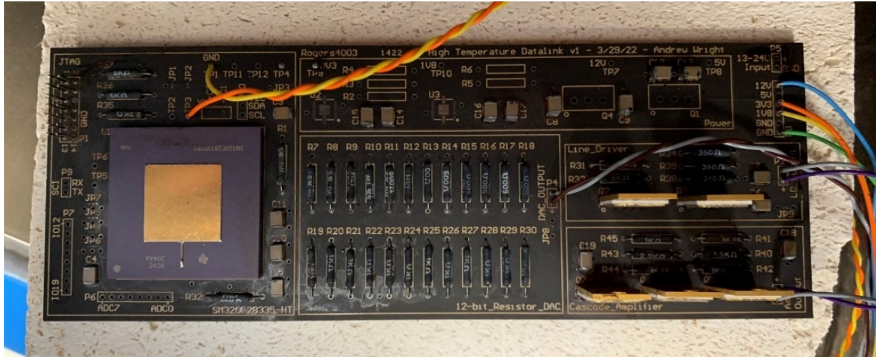
Figure 34. The data link after operating at 210°C for 288 hours.
