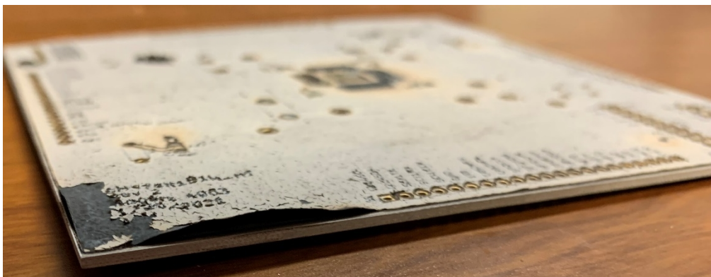
Figure 13. Degradation of PCB at 300°C. Solder mask changed from a green to a white color and delaminated from the Roger4003 material. The board planarization also degraded and was no longer flat.
