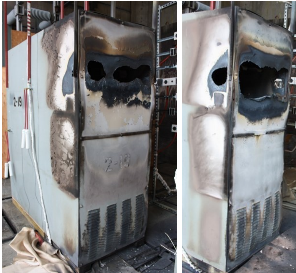
Figure 6. Photographs of 2 sec test enclosures (Left 2-19 25.8kA 39MJ / Right 2-22 32.0kA 51MJ)
