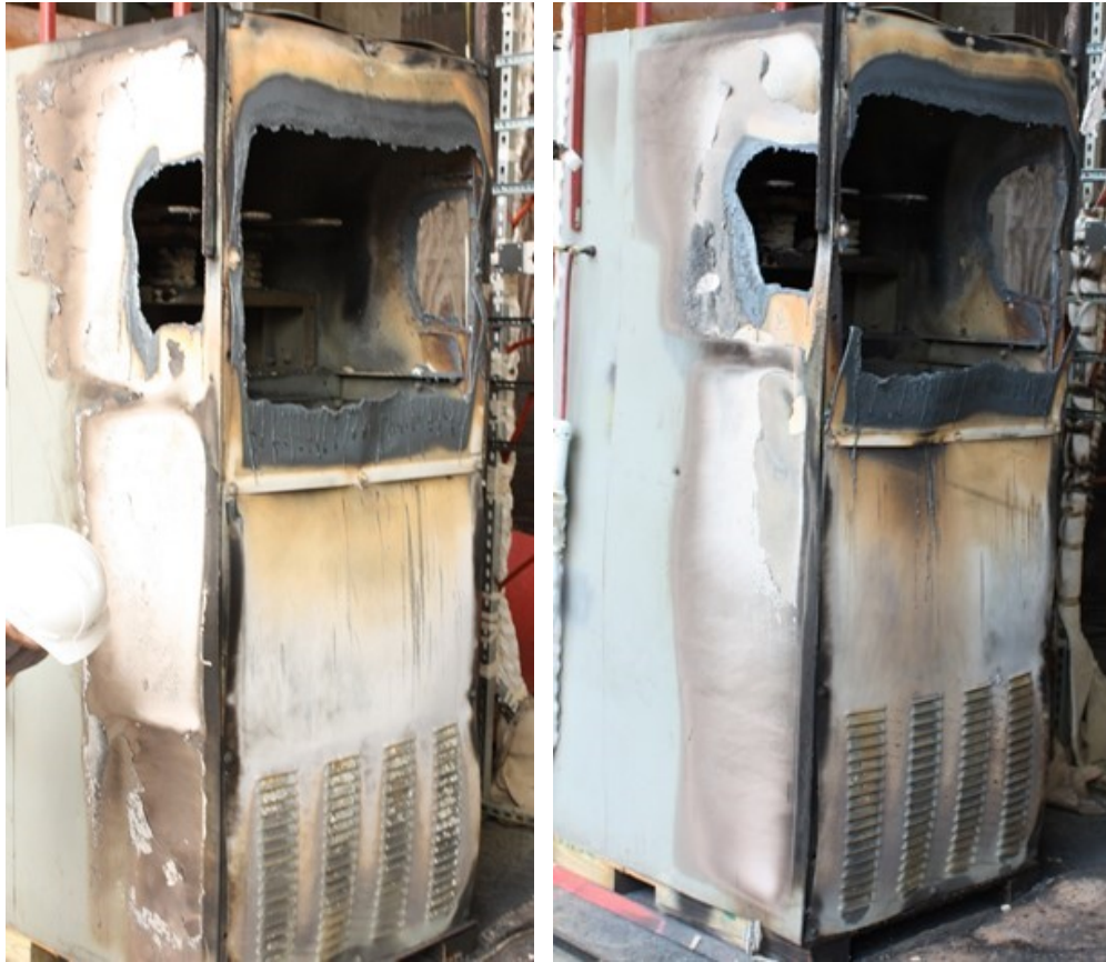
Figure 7. Photographs of 4 sec test enclosure (Left 2-21 26.6kA 101MJ / Right 2-24 29.8kA 122MJ)
