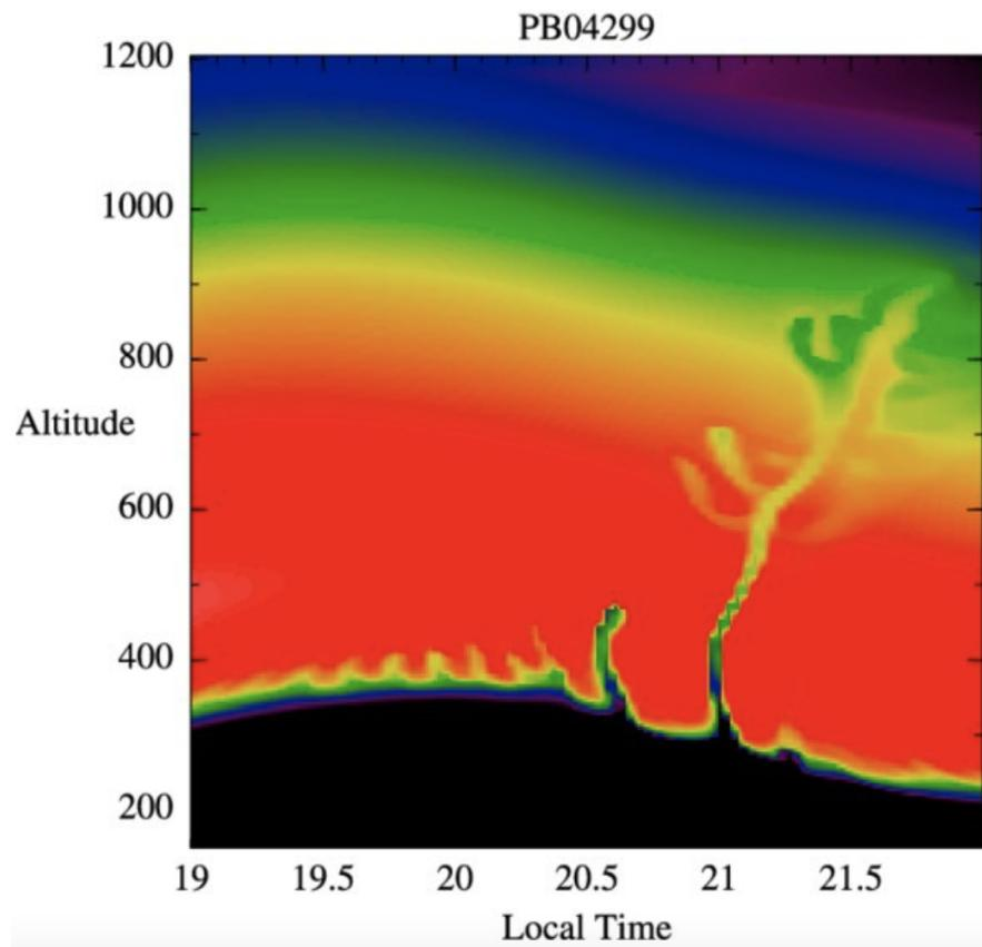
Model for a naturally occurring ionospheric electron density “plume”.
