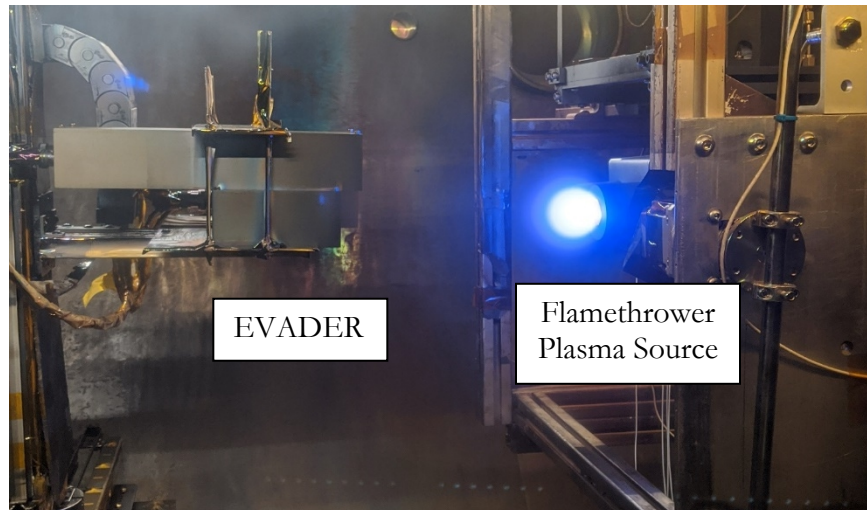
Figure 2. The EVADER probe is aligned with the Flamethrower 25cm away, collecting steady-state data on a krypton plasma.
