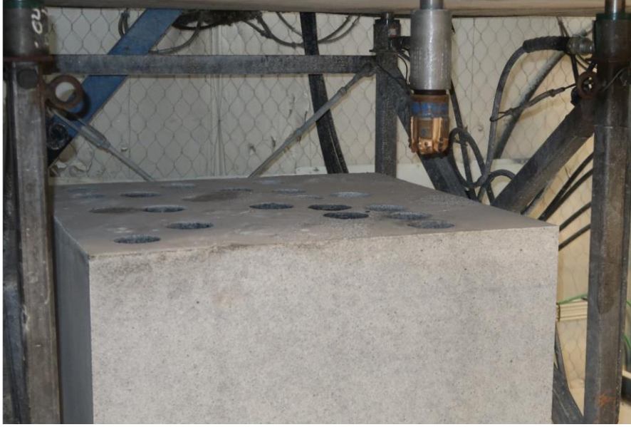
Figure 3: Photograph of Sandia’s Hard Rock Drilling Facility.
