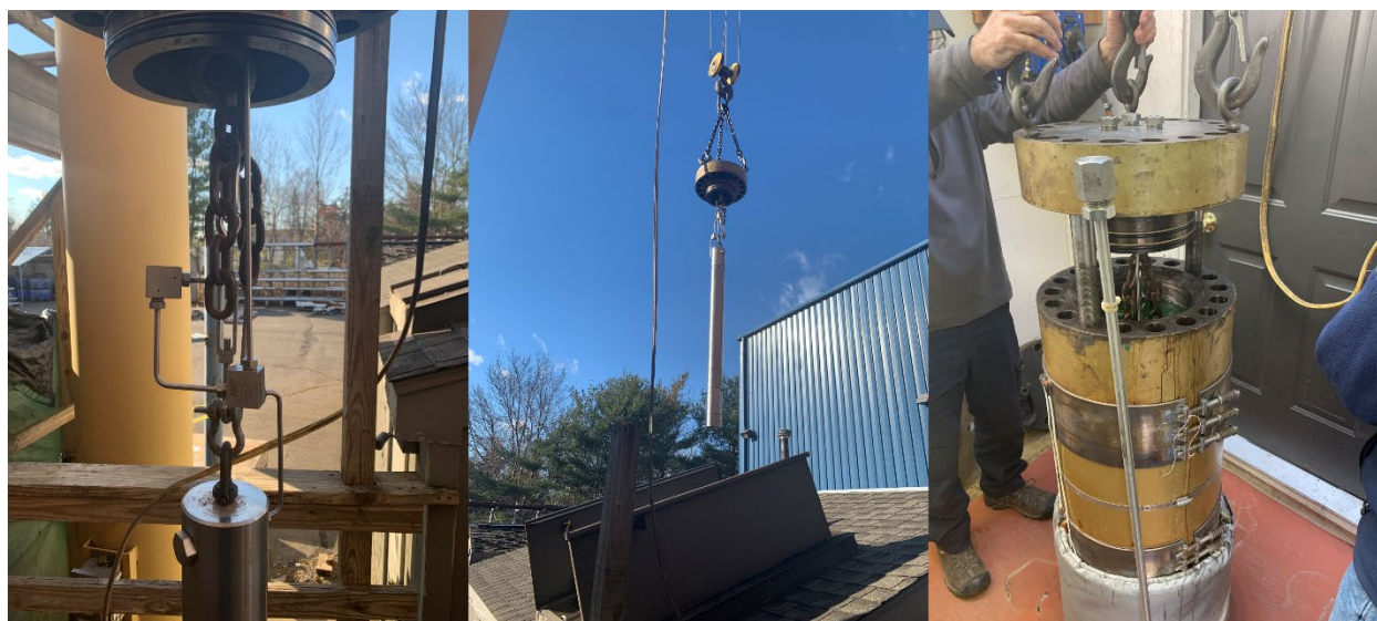
Figure 5-11. From left: The TEG tool shown attached to the top closure of the pressure vessel at APS, showing the high-pressure piping used to produce the high internal pressure in the tool; top closure hoisted by a crane and inserted into the top of the building used to house the large pressure vessel at APS; top closure at attached tool being lowered into the pressure vessel at APS prior to pressure testing and heating.
