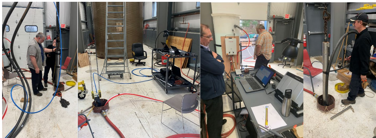
Figure 5-6. From left: Lowering the renewed tool into the experimental wellbore; Hot and cold hoses inside the wellbore at lower left; APS staff monitoring the thermocouple response (foreground) and heater temperature (background); extracting the tool at the end of the test.
