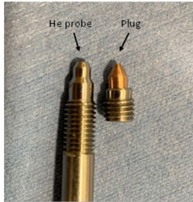
Figure 5-3. Comparison of the He probe tip and the He port plug. The tapped threads had to be extended deeper into the port for the plug to properly seat and seal the port.
