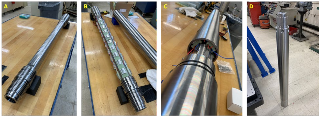
Figure 4-5. Preliminary assembly of field prototype energy harvester to test clearances. A) Bare inner assembly. B) Inner assembly with TEGs and thermal bridges in place. C) Sliding the outer shell the thermal bridges. D) Unit with outer shell fully in position.
