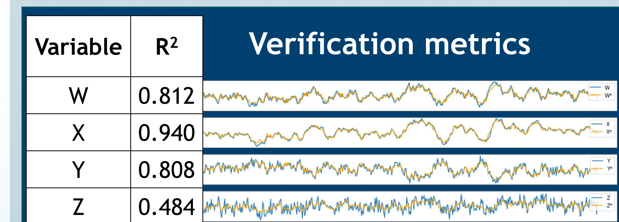
Example of a verification metric to determine if our directed graphs are trustworthy in the absence of ground truth. In this case we are checking to see if the RFR can predict our data well
