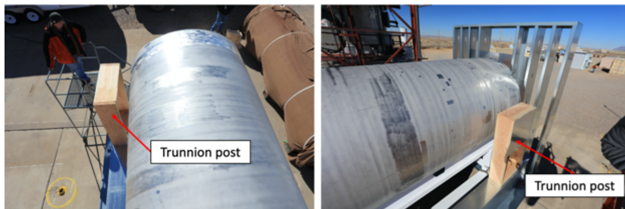
Figure 3.7 The canister on the transfer skid and the location of the trunnion posts.
