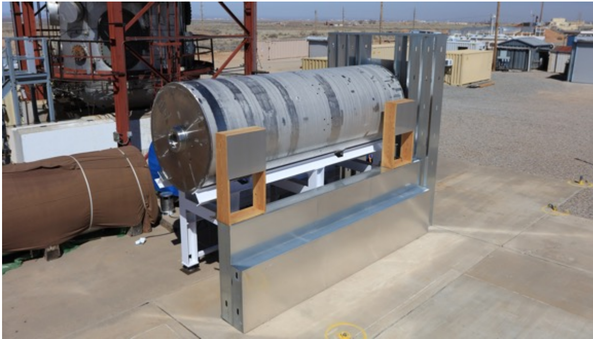
Figure 3.3 Transfer skid mockup and canister at the Surtsey site located in Tech Area III of Sandia National Laboratories.
