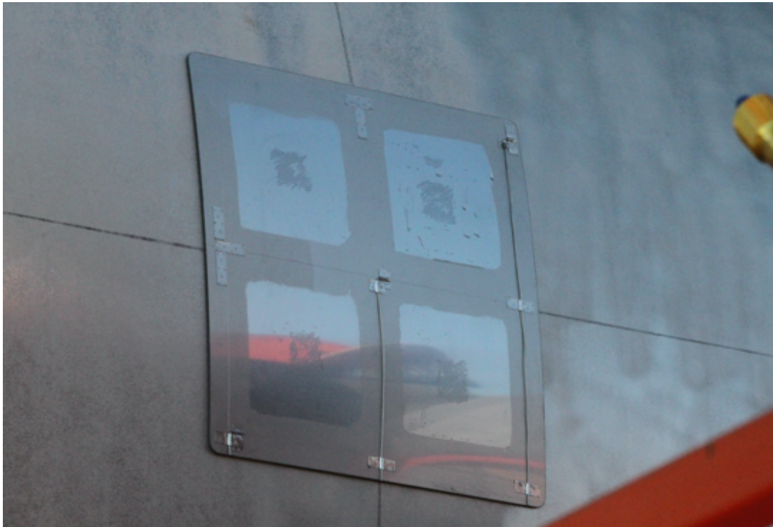
Figure 3.22 A picture showing sample plate 3 after all quadrants were sampled. It is clear from this picture that some water and possibly salt was left behind on 3B.
