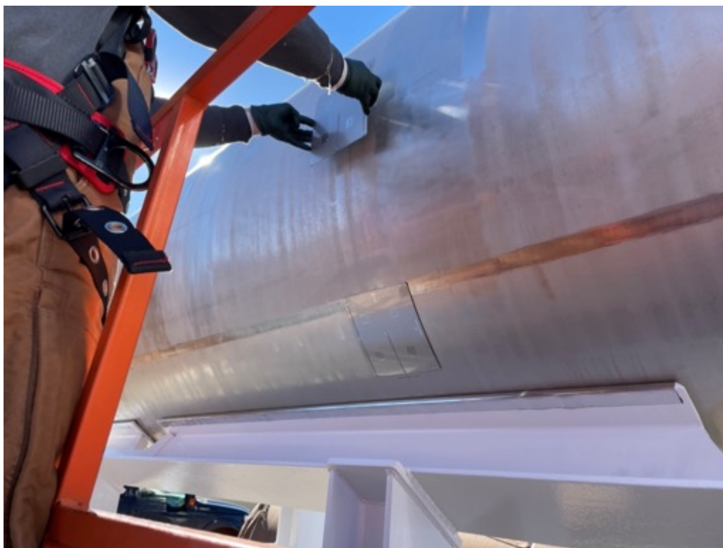
Figure 3.14 Sampling plate placement on canister surface at position W3 with plate already positioned at W4.
