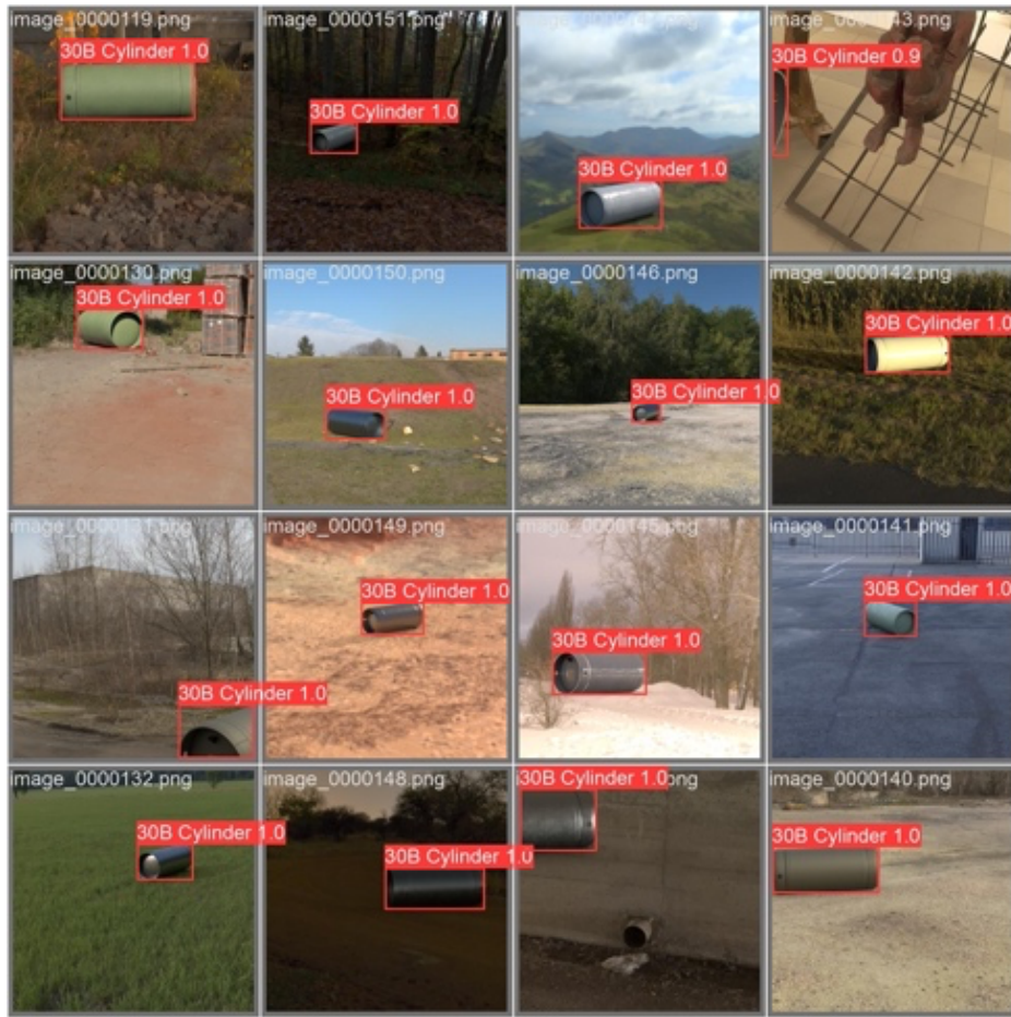
Figure 5: Preliminary training accuracy of YOLO_v5 for containers.
