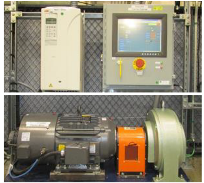
Fig. 3. Diesel generator emulator and dual-wound generator (bottom), drive and controller for diesel emulator shown above
