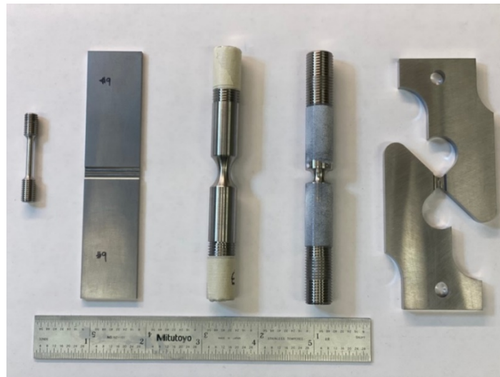
Figure 1. Test Specimen Geometries (Left to Right: R5, Flat-Groove, 9 mm Notch, 3 mm Notch, and Shear).
