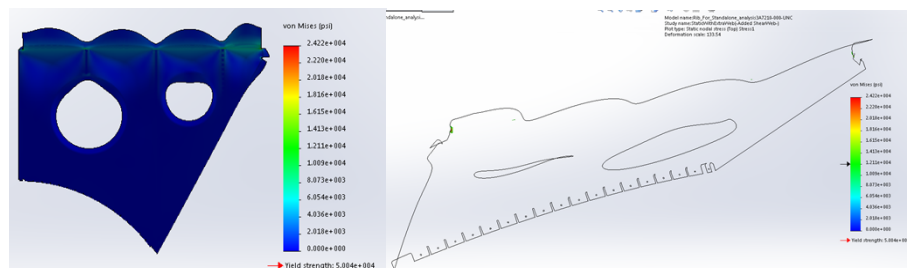
Figure 9: Deformed plot of primary stress and deformation of the flange area, scale is 133:1 right side shows the small areas subjected to stresses above 82.7 Mpa
