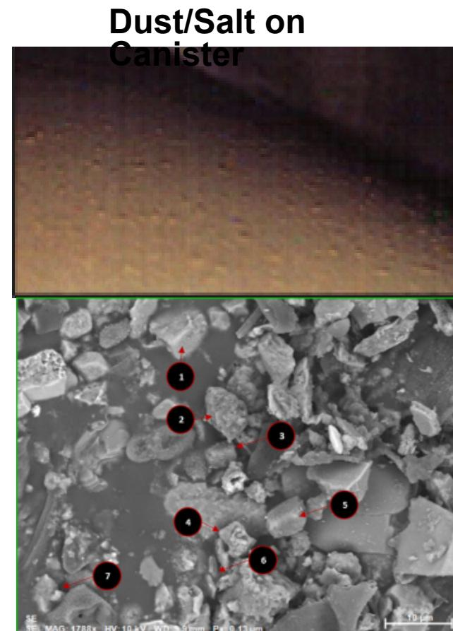
As canister cools, salt and dust is deposited on canister
