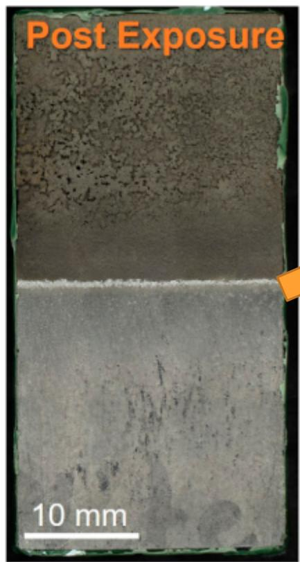
Undercutting after Ferric Chloride Testing
