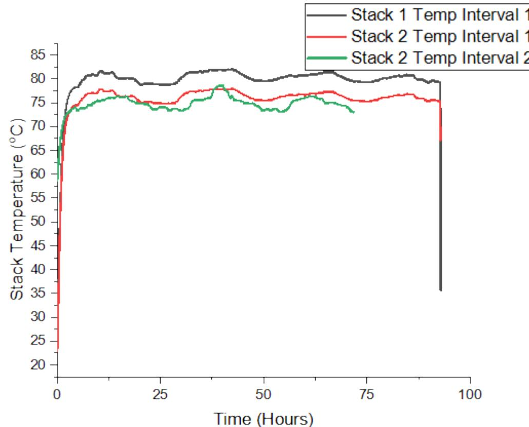
Coupons were stacked and layered in aluminum foil prior to loading in the shutter array. These stacks had a large volume which self-heated in the high flux of the shutter array.
