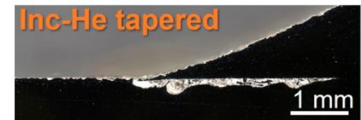
In accelerated ferric chloride tests, factors such as the surface roughness, coating porosity, the interface type (tapered or masked) and the amount of deformation in the substrate influenced the corrosion behavior of the cold spray. Careful alloy selection did not eliminate corrosion in accelerated testing.
