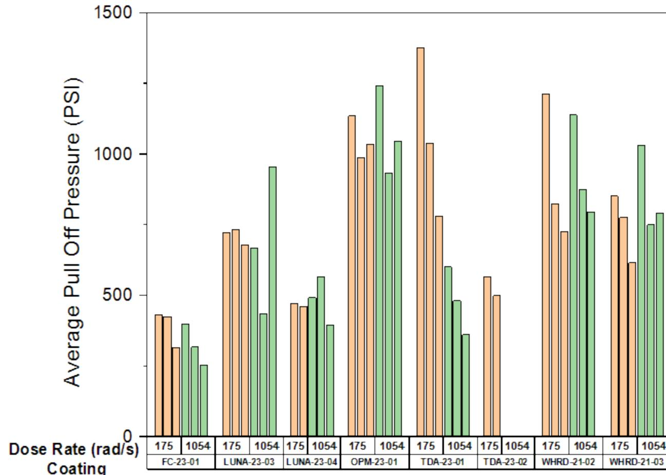
Actual max dose rate on loaded canister is 2-3 rad/s, used 175 rad/s and 1054 rad/s in these tests. Further investigation on implications of dose rate effects are ongoing.
