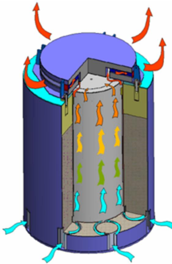
Canister is passively cooled, convection pulls in ambient air (occurs in horizontal and vertical storage systems)
