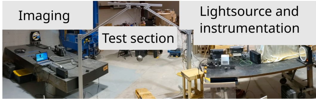
Figure 2.1: Alignment setup for Z-type schlieren
