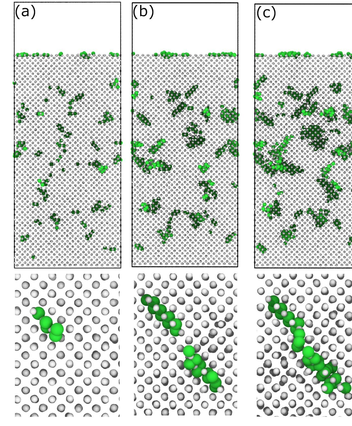
Atomistic snapshots of hydrogen (green) implantation in tungsten (grey) at (a) 5 ns, (b) 10 ns, and (c) 15 ns. Bottom images depict the growth of one platelet in the simulation.
