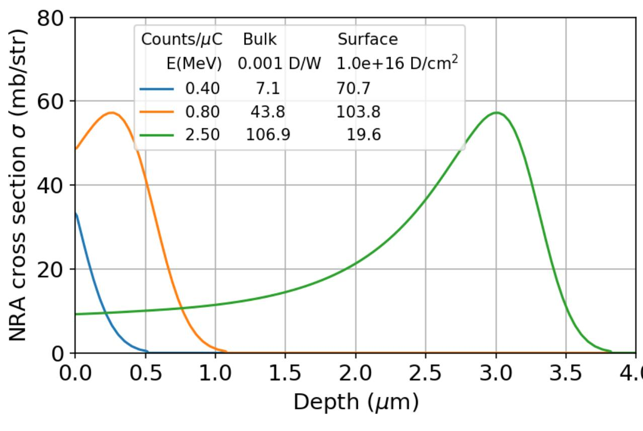
Can distinguish bulk D from surface D from yield vs  $\text{He}^3$  energy:
