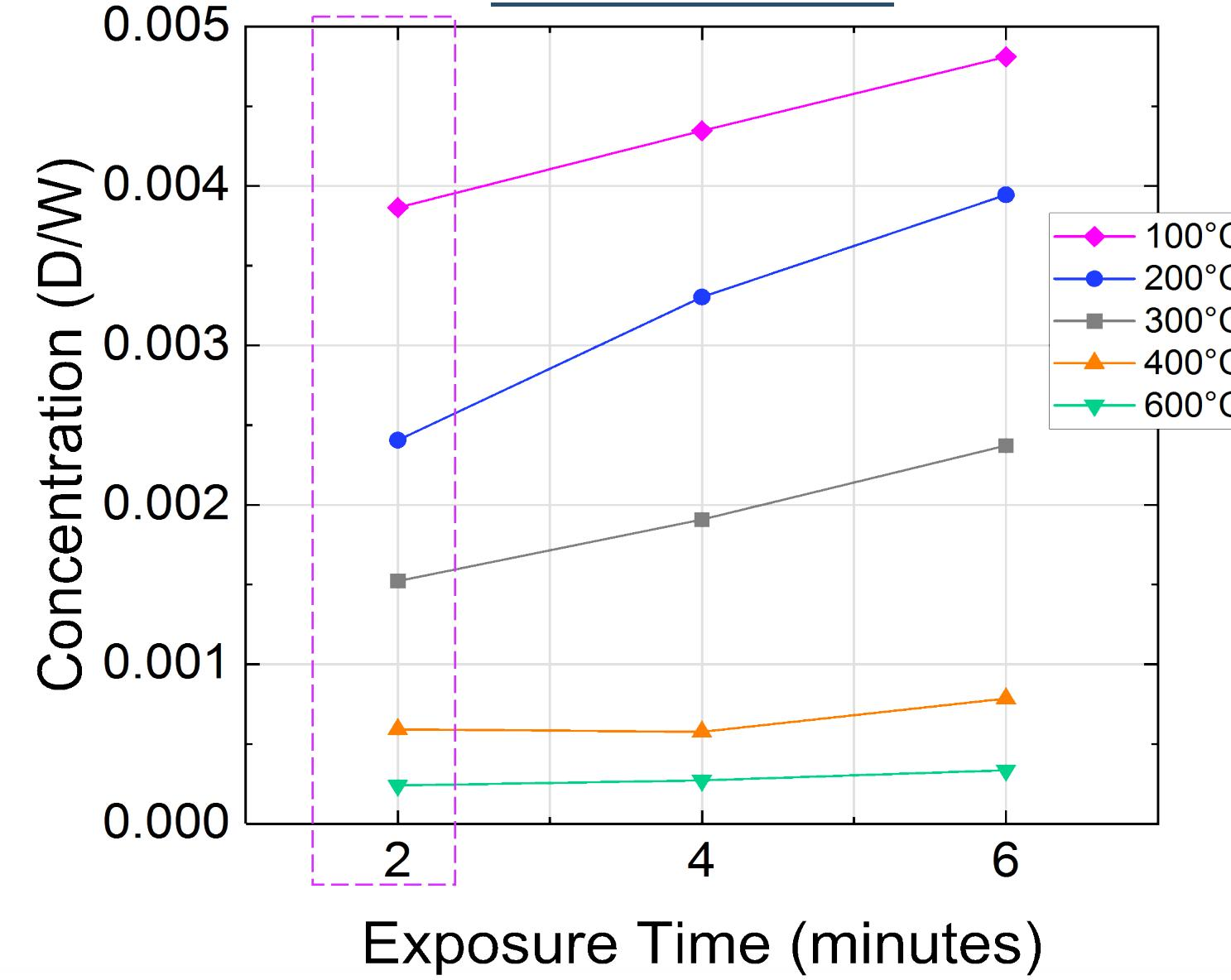
We observed evidence of temperature dependent deuterium retention. As temperature increases, the near-surface retained deuterium decreases. The deuterium decrease is even more prominent at high temperature where there is little to no significant retained deuterium changes from 2 minutes to 6 minutes.
