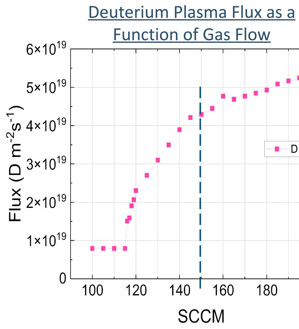
Flux quickly increases as a function of gas flow (between 110 sccm to 140 sccm) and then tapers off. As a result, 150 sccm gas flow was chosen during experiments.
