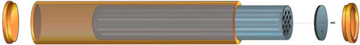
Figure 3-3. Exploded view of the canister components (from left: copper base, copper tube, insert, steel lid for insert and copper lid) (from SKB 2011, TR-11-10).
