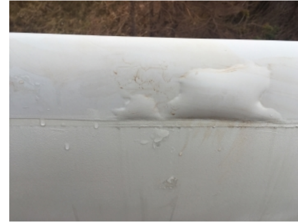
Conventional leading edge erosion protection tape
