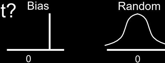
Bias errors will probably be from differences in inflows if measurements are not simultaneous and more or less co-located and from any differences in the turbines if we use two. Bias errors may be mitigated by binning data to compare similar conditions.
