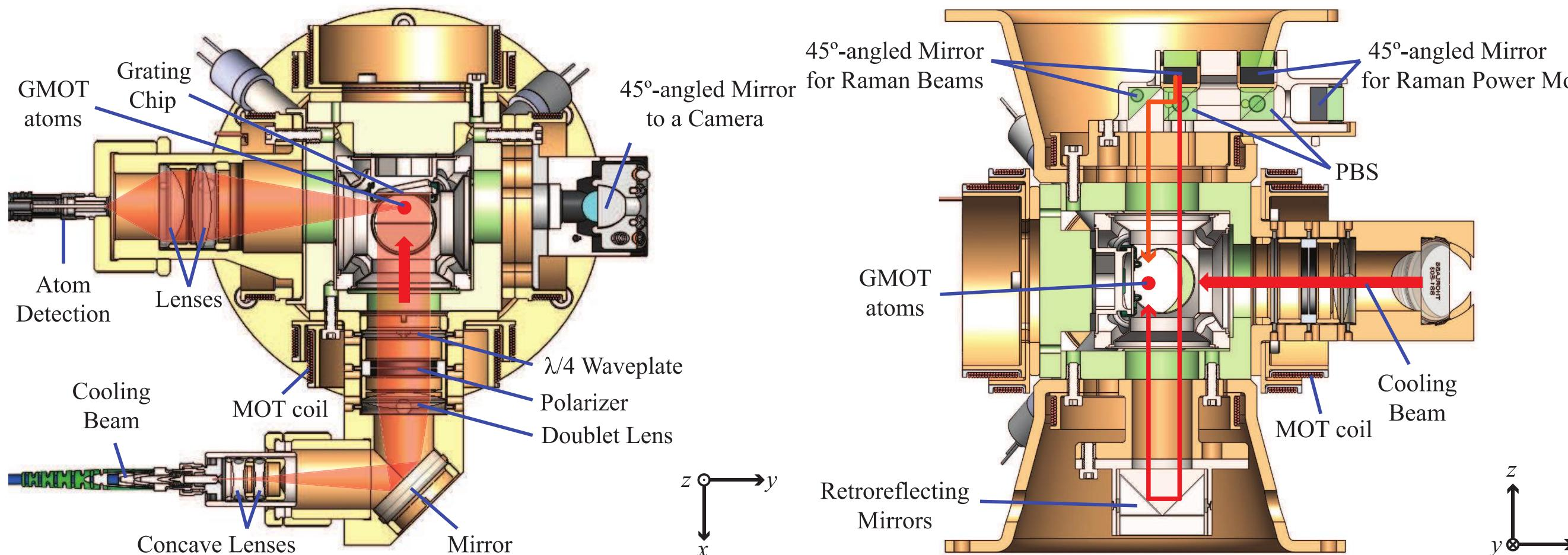
**In-house-fabricated grating chip** is composed of three binary gratings in a triangular orientation to form a tetrahedral GMOT [4-6].
