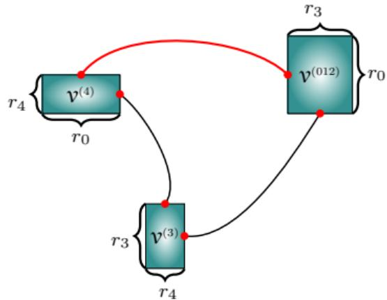
Full tensor network contraction consists of a set of recursive pairwise contractions until one vertex is left
