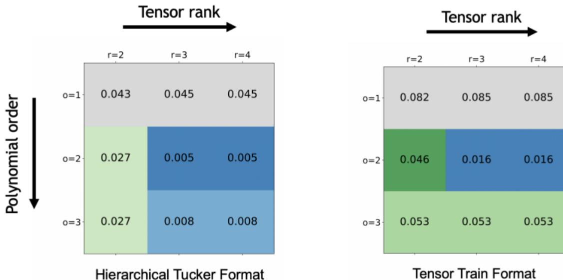
Site US-Ha1/June: Validation mean-squared error for Hierarchical Tucker models compared to Tensor Train models
