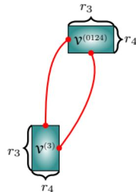
Full tensor network contraction consists of a set of recursive pairwise contractions until one vertex is left
