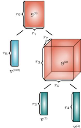
*Full tensor network contraction consists of a set of recursive pairwise contractions until we exhaust all connections*
