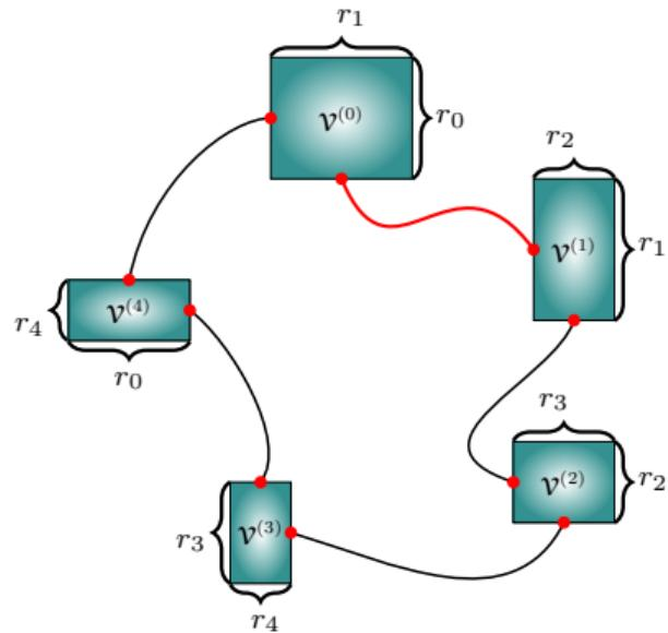
Full tensor network contraction consists of a set of recursive pairwise contractions until one vertex is left
