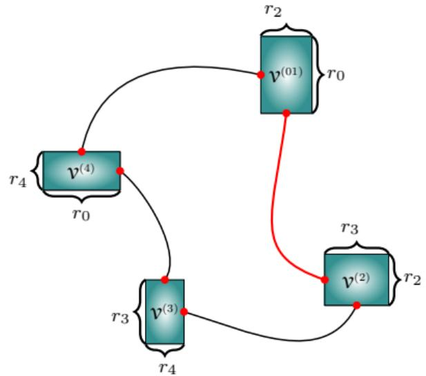
*Full tensor network contraction consists of a set of recursive pairwise contractions until one vertex is left*
