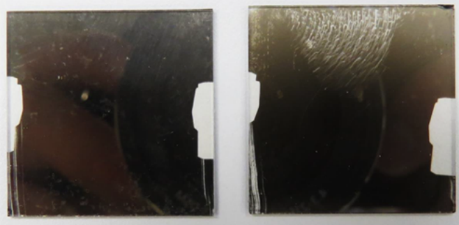
Glass slip after laser milling
