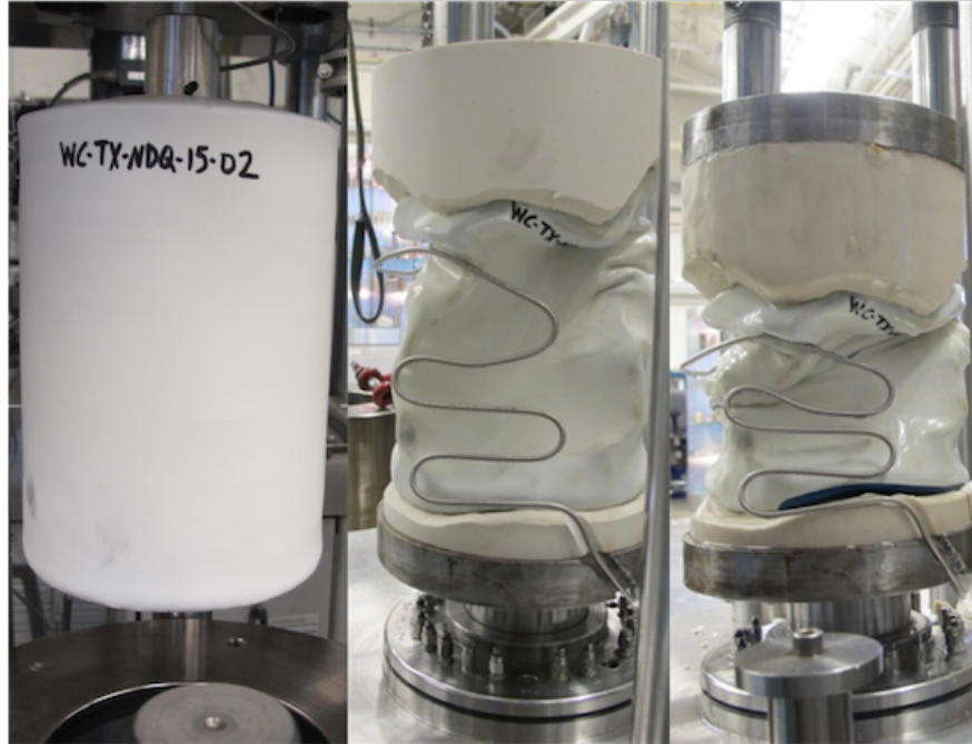
Figure 2-18. Specimen WC-TX-NDQ-15-02 before compaction (left), after hydrostatic compaction at 15 MPa and with Hydro-Stone® formed endcaps molded on (middle), and after 27% axial strain during triaxial compression (right). Upper and lower steel endcaps are visible.
