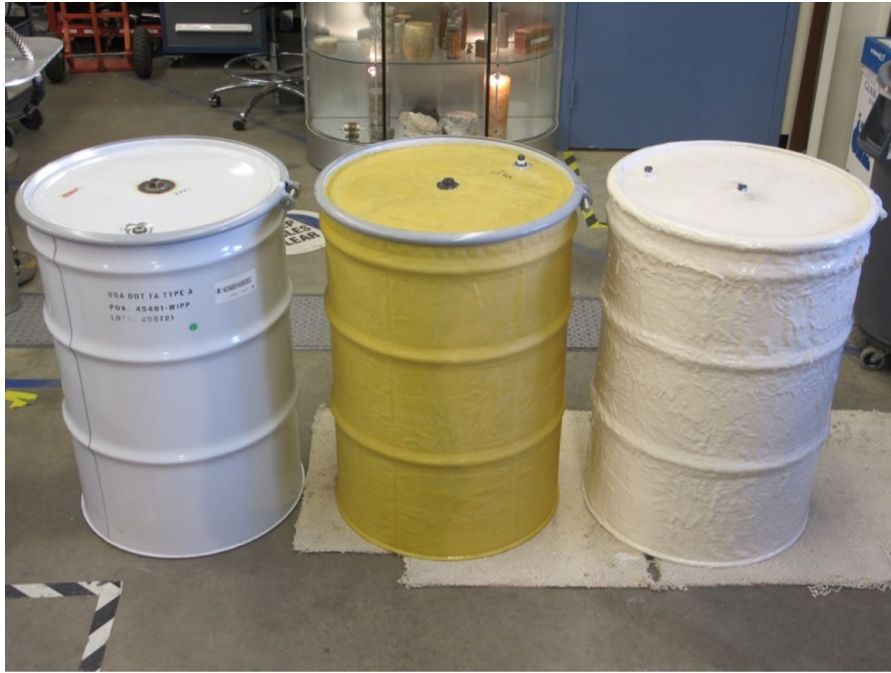
Figure 2-22. Photographs of the jacketing process for full-scale drums to be tested under hydrostatic conditions. A new drum with no jacketing (left), a drum wrapped in Kevlar® and coated with one layer of PMC®-770 (center), and a finished sample with multiple coats of Brush-On®-40 applied (right).
