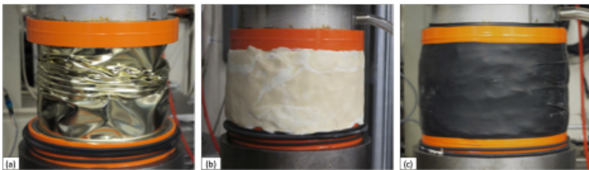
Figure 2-10. Photographs of the jacketing of a 1/4 -scale uniaxial test specimen WC-UC-NDQ-10. (a) The sample is loaded until the can was breached. (b) The sample was covered in modeling clay. (c) The rubber sleeve was pulled up over the clay and tightly taped around the upper and lower platens to seal it.
