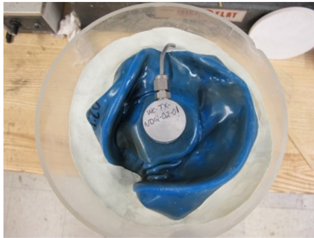
Figure 2-17. Photograph of a pre-compacted sample in the acrylic mold with a vent port and flexible tubing attached to vent nipple on top of specimen. The white material below the sample is Hydro-Stone® gypsum cement.
