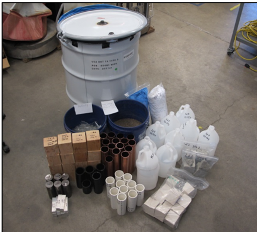
Figure 2-1. Photograph of surrogate waste components used in a full-scale 55-gallon drum.
