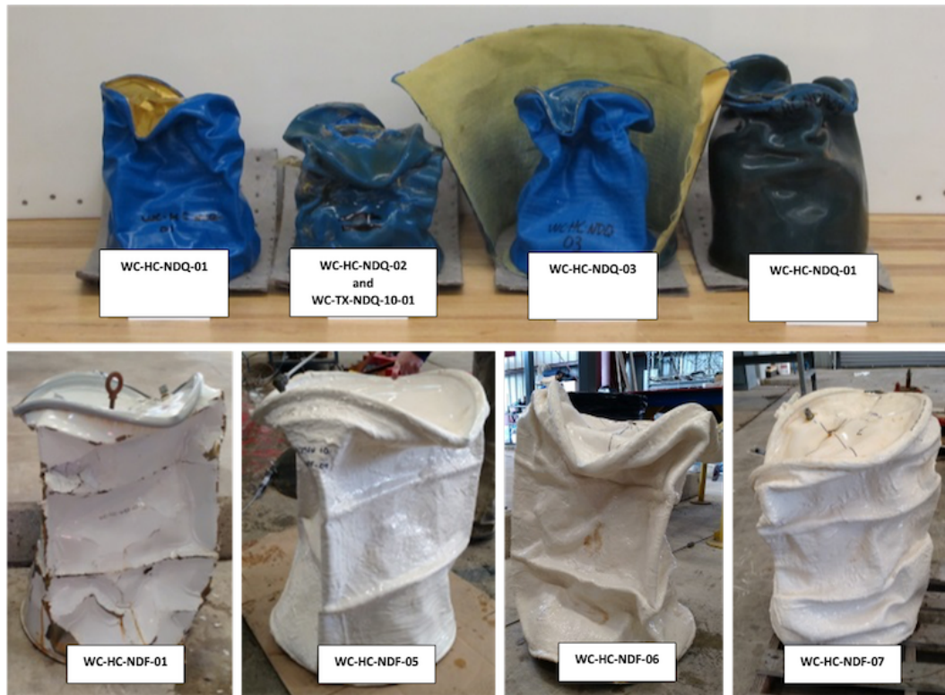
Figure 2-26. Photographs of 1/4 -scale (top row) and full-scaled (bottom row) post-test hydrostatically compacted samples.
