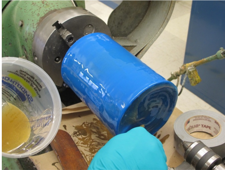
Figure 2-24. Photograph of a 1/4-scale hydrostatic sample being coated with PMC ® -770 urethane rubber over the three coats of Loctite ® SF F720 and two layers of Kevlar ® sheets.
