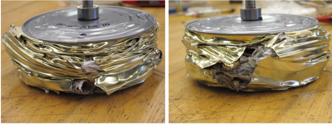
Figure 2-9. Photographs of specimen WC-UC-NDQ-10 at the end of its test. The sample shows numerous large splits in the sample's side which occurs underneath the clay and rubber sleeve jacket.
