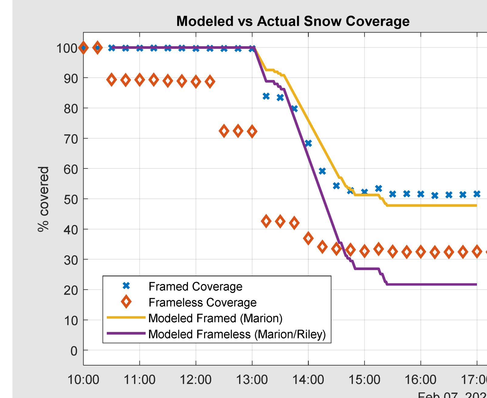
In 25% of cases where the actual shedding rates of framed and frameless modules differed, the framed PV modules shed more quickly. In these cases, the modified model caused larger errors than the standard model.
