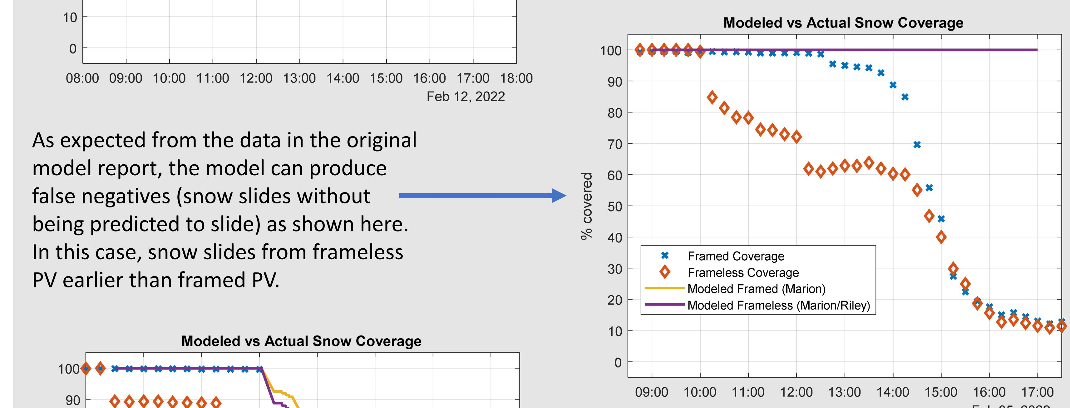
In 75% of cases where the actual shedding rates of framed and frameless modules differed, the frameless PV modules shed more quickly. The modified model accurately reflects this faster shedding.
