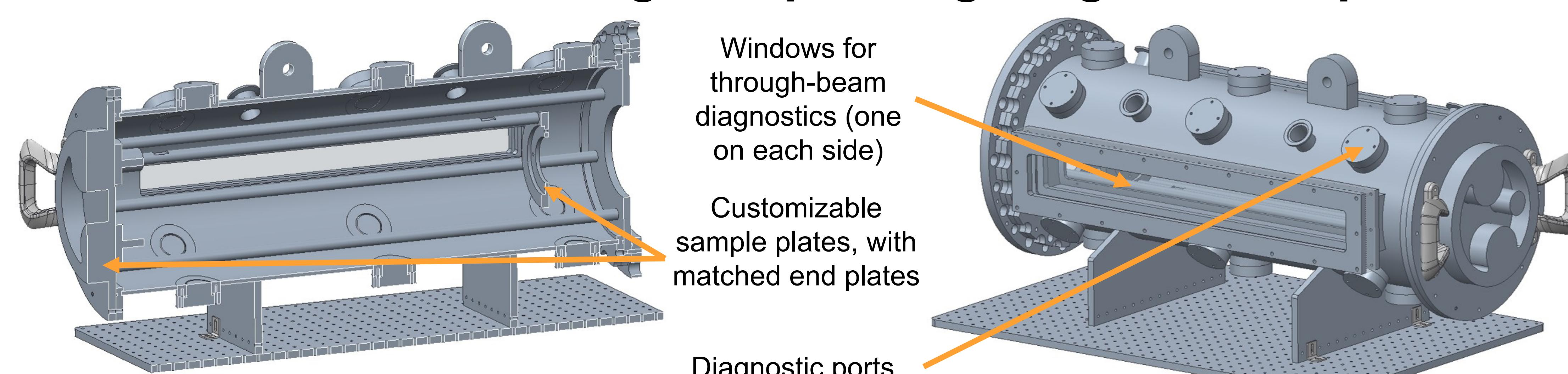
Diagnostic capabilities that are being planned for use with the new gas cell:
