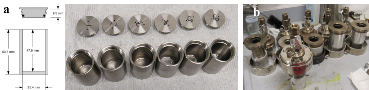
Figure 2: Equipment used for hydrothermal experiments involving produced microcapsules and sodium silicate solutions. To minimize fluid loss and chemical contamination of the samples, sealable internal cells (a) were used in combination with small Parr reactor vessels (b). These vessels were heated in a convection oven at 150-200 °C (From Nakagawa et al., 2022).
