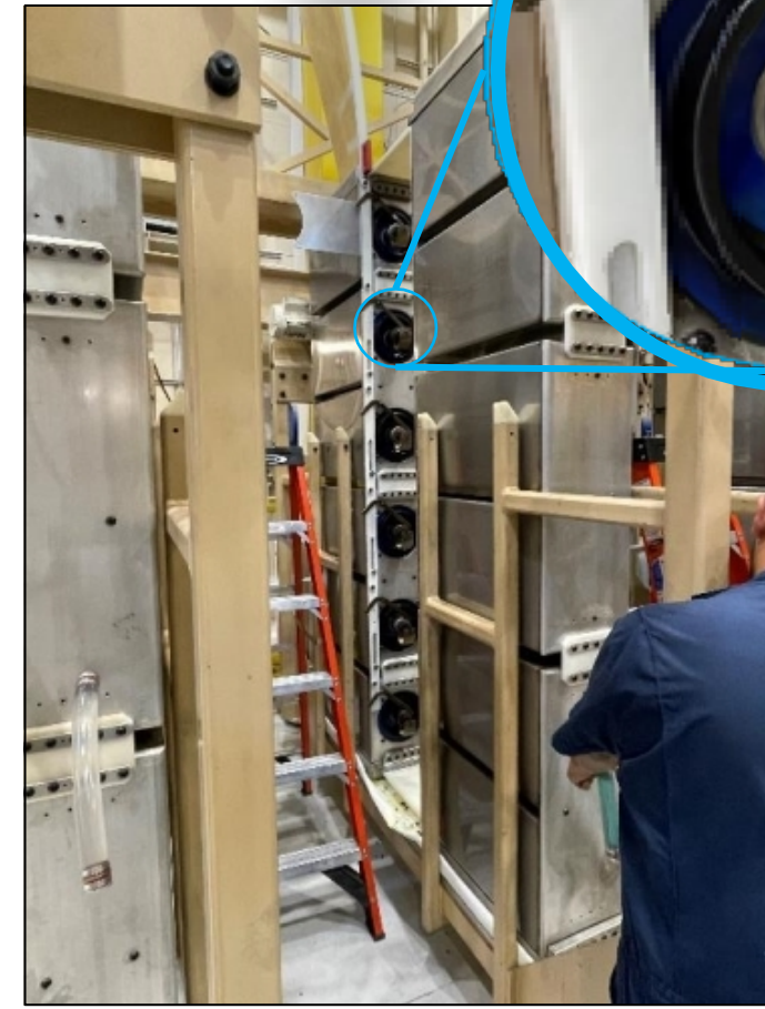
Spring loaded shorting arms are employed to dump energy in oil tank; jumper bar locked in SHORTED position during maintenance
