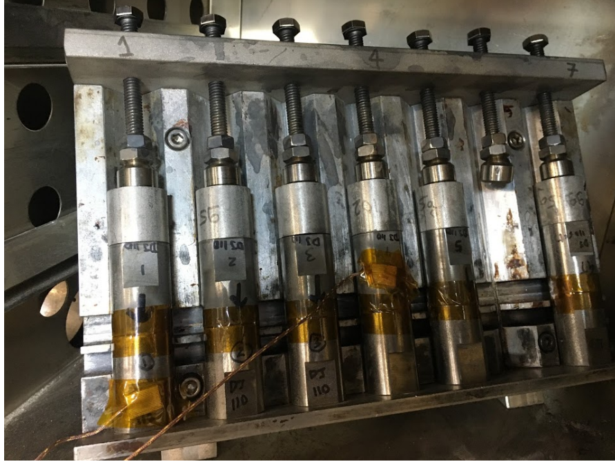
Figure 12. Slug and sample fixture for furnace curing
