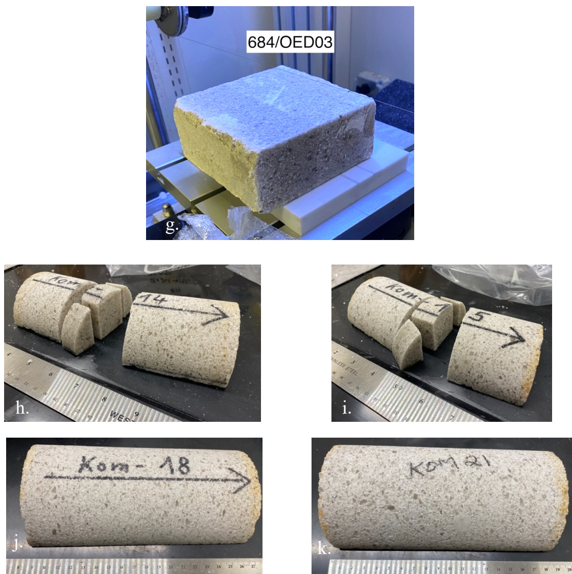
Figure 1. Reconsolidated granular salt samples from oedometric tests at IfG (parts a through g) and triaxial tests at TUC (parts h through k)
