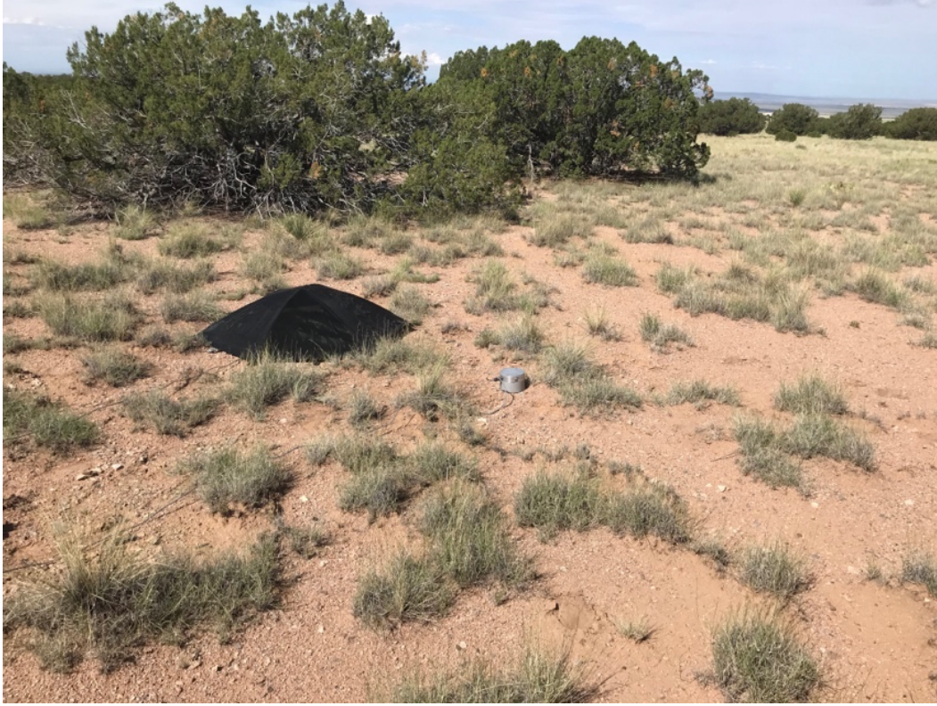
Figure 2. Co-located infrasound sensors with (right) and without (left) the trampoline fabric wind filter.
