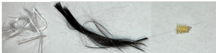
Figure 2-1. From left to right: glass fibers, carbon fibers, cut sample of epoxy, all before decomposition.
