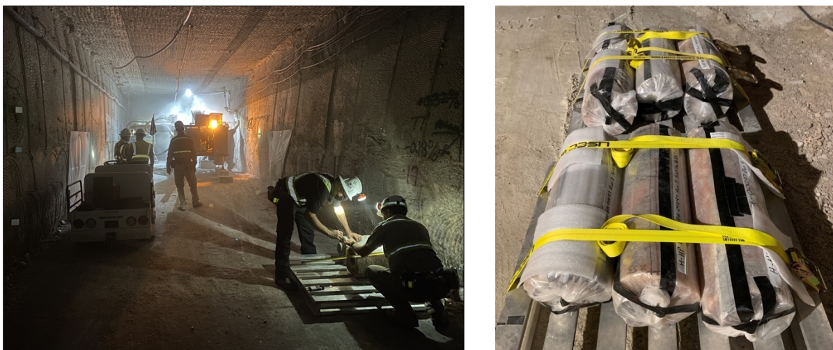
Figure 4. BATS-1 over-coring; left: WIPP TCO processing over-core, right: over-core on pallets.
