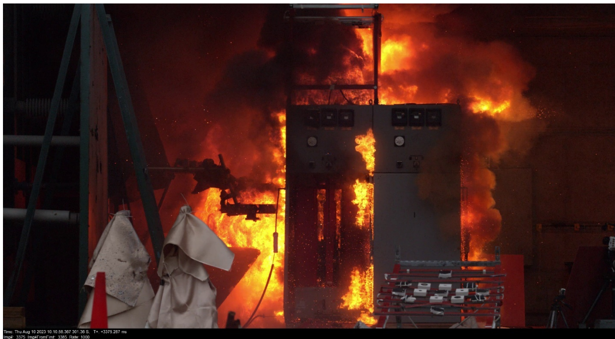
Figure 3-13: Test 2-37 imaged through 4k camera 3 second into the test – camera imaging at 1000 fps – where the arc is affecting the second enclosure (mostly in the back). Notice the instrument stand on the ground by this time.
