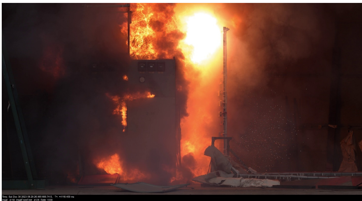
Figure 3-44: Test 2-39 imaged through 4k camera 3 seconds into the test – camera imaging at 1000 fps – showing the instrument stand on the ground and the burning in the back of the southeast and northeast enclosures. The southeast enclosure also shows fire coming out from one of its access door.
