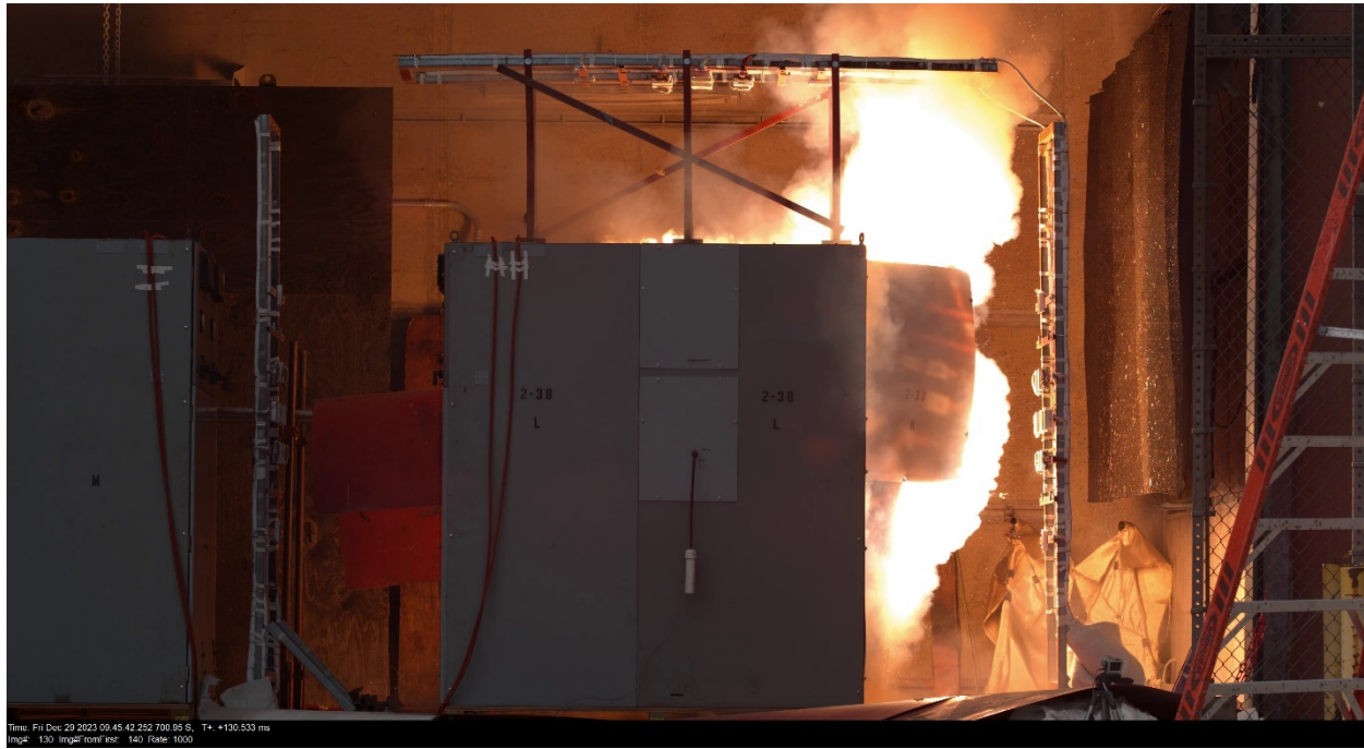
Figure 3-30: Test 2-38 imaged through 4k camera – camera imaging at 1000 fps. Notice the panel ejected to the east. The arc was initiated in the north enclosure – behind the enclosure in view.
