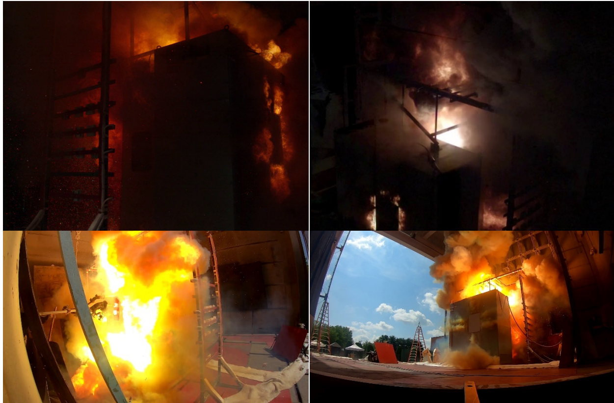
Figure 3-24: From top left (clockwise): v1310 view at 1.5 seconds into the test while venting in the adjacent enclosure; v7 elevated from the northeast of the test while the east side enclosure vents but the arc starting enclosure suffers the brunt of the test; GoPro outside west during the arc on the west side enclosure; GoPro inside floor northeast view of the damage to the first enclosure while the second enclosure starts venting gases.
