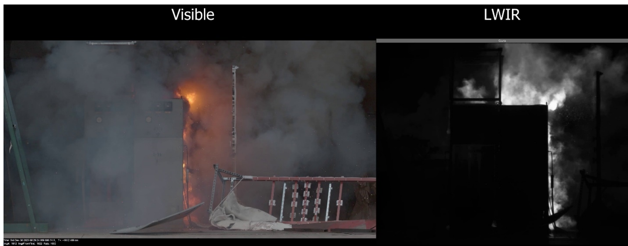
Figure 3-47: Sample frames from synchronized video of 4k and LWIR cameras close to 1.5 seconds into the test. The LWIR image shows heat (probably fire) at the interface between the north and south enclosures and that part of it is occluded by the smoke.
