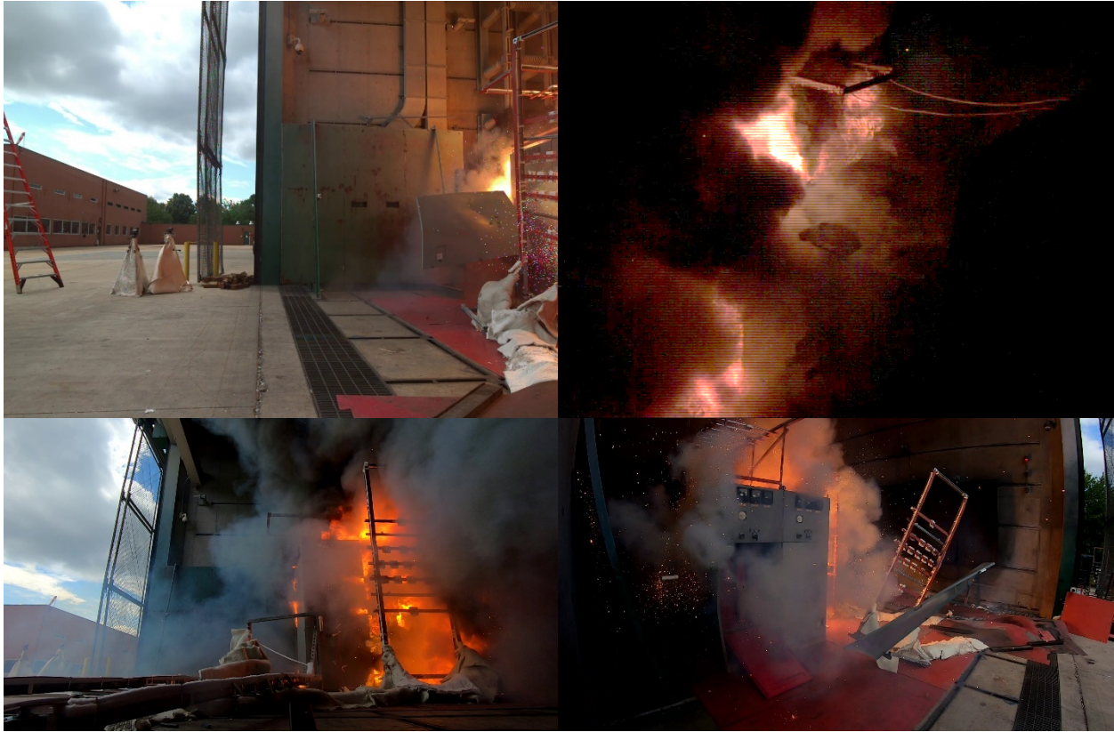
Figure 3-45: From top left (clockwise): v1310 view 0.25 seconds into the test with the access door twirling away from the enclosure; v7 elevated from the northeast of the test bay, at 2.5 seconds, while showing fire at the interface of the southeast and northeast enclosures; GoPro inside floor southeast view showing instrument stand in the ground and the southeast enclosure east side ejecting fire during the test; GoPro southwest view while instrument stand and door enclosure fall to the ground.
