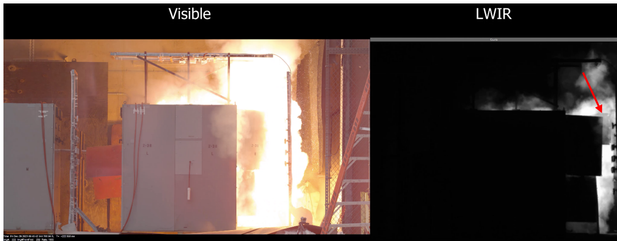
Figure 3-37: Sample frames from synchronized video of 4k and LWIR cameras at the beginning of the test. The LWIR image shows the square profile of the panel ejected from the enclosure where the arc was started, see red arrow.
