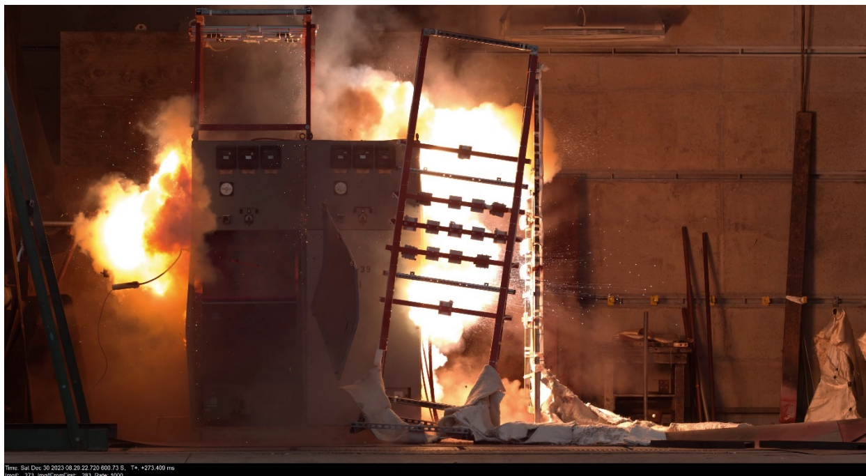
Figure 3-43: Test 2-39 imaged through 4k camera 230 ms after the previous image in Figure 3-40 – camera imaging at 1000 fps – showing multiple explosion while the rack is falling.
