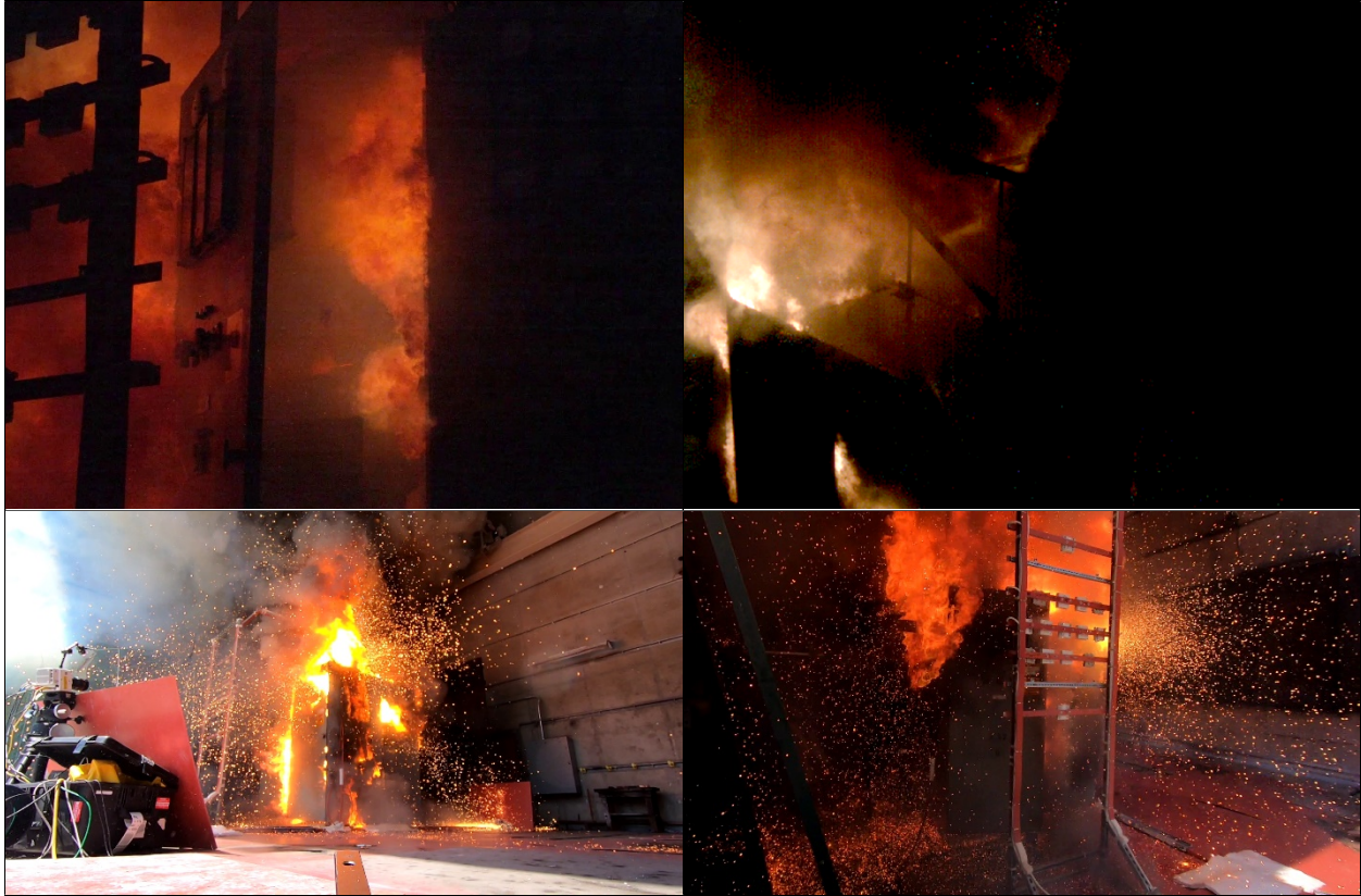
Figure 3-5: From top left (clockwise): v1310 while the door is being blown open; v7 elevated from the northeast of the test while the east side enclosure vents; GoPro outside southwest; GoPro outside floor southeast while molten material is dumped out of the east enclosure.
