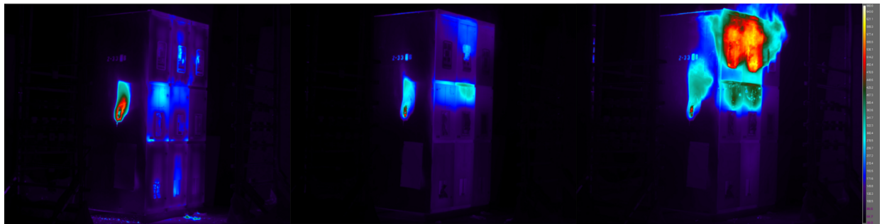
Figure 4-15: Temperature images from the LWIR camera A655 through 8.5 minutes intervals, starting right after the test. Arc is induced in the west most enclosure (red hot on top). Temperature ranges from 38.9 to 660°C.
