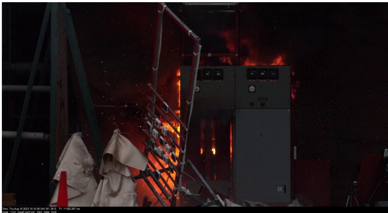
Figure 3-12: Test 2-37 imaged through 4k camera 1 second into the test – camera imaging at 1000 fps – where the instrument stand is falling after being pushed by the ejected door from the enclosure where the arc is initiated.
