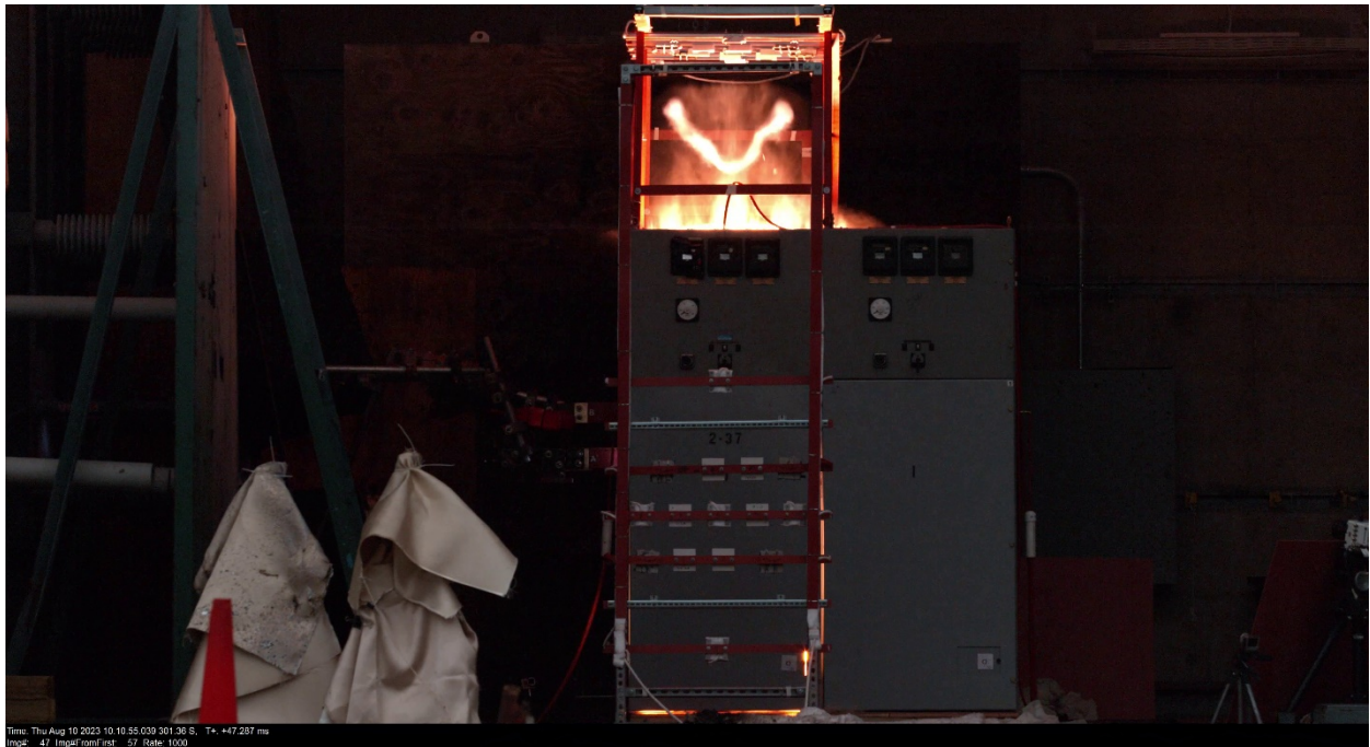
Figure 3-11: Test 2-37 imaged through 4k camera first millisecond into the test – This camera imaging at 1000 fps – showing a v-shape object being ejected on the top.
