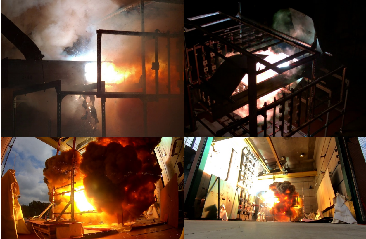
Figure 2-5: From top left (clockwise): v1310 at southwest side showing the enclosure being consumed by the arc; v7 elevated from the northeast showing the initial breach; GoPro outside southeast; GoPro inside floor northeast.
