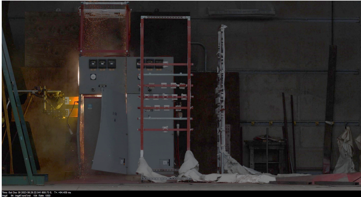
Figure 3-41: Test 2-39 imaged through 4k camera 46 ms after the previous image in Figure 3-40 – camera imaging at 1000 fps – showing access door being ejected and deforming.
