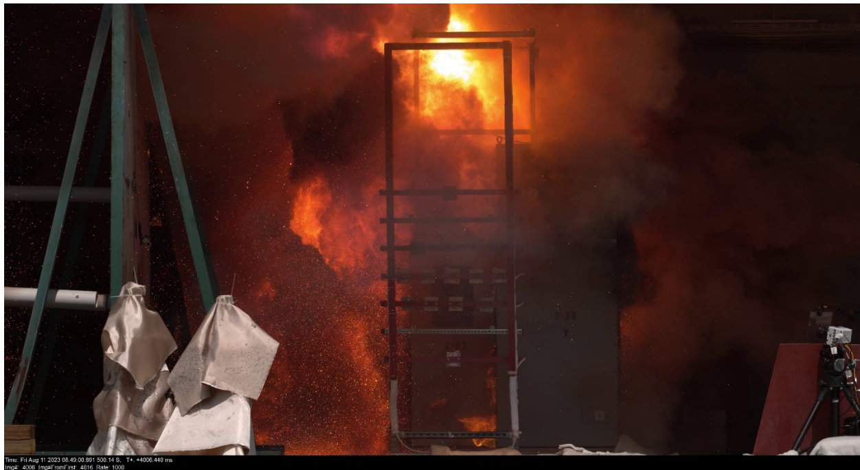
Figure 3-23: Test 2-36 imaged through 4k camera – camera imaging at 1000 fps – 4 seconds into the test. There is a fire engulfing the enclosure where the arc was initiated, also there is spray of burning metal particulate. The second enclosure seems to be mostly engulfed by the dark smoke with some fire activity on the east side.
