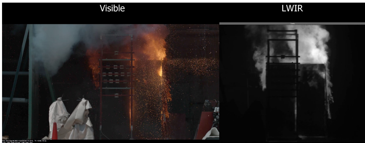
Figure 3-8: Sample frames from synchronized video of 4k and LWIR cameras 3 seconds into the test. Notice that the IR doesn't show the metal spray to the right of the second enclosure. The spray of metal particulate that probably emitting light in the visible in a narrow band instead of the continuum from a Planck curve profile.
