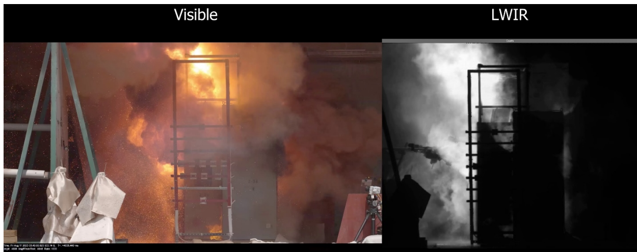
Figure 3-27: sample frames from synchronized video of 4k and LWIR cameras close to 4 seconds into the test. While there seems to be activity in IR and visible in the back (north side), the IR seems to indicate that the second enclosure is not that hot, even if the first enclosure keeps burning for several minutes after the test.
