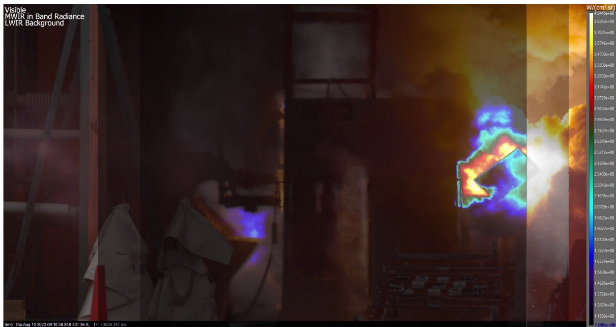
Figure 3-17: Image fusion of IR camera (in radiance units of W/cm 2 sr) synchronized with a visible image almost 4 seconds into the test showing the ejection of a panel of the adjacent enclosure.
