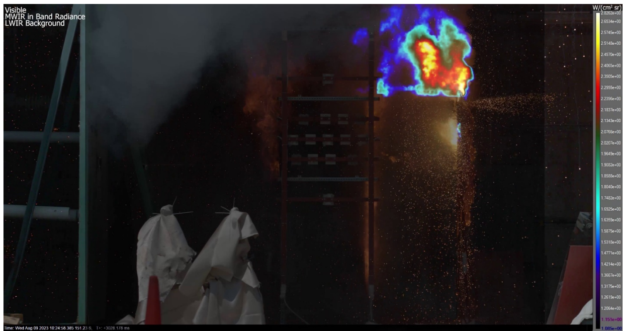
Figure 3-7: Image fusion of IR camera (in radiance units of W/cm 2 sr) synchronized with a visible image 3 seconds into the test. Notice that the higher fire activity is occurring on the adjacent enclosure.
