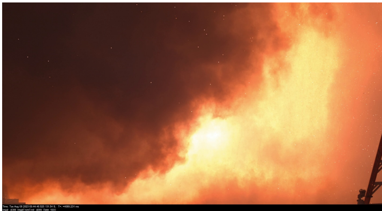
Figure 2-12: Test 2-41 imaged through 4k camera – camera imaging at 1000 fps. Notice that a dark cloud envelopes the test bay 4 seconds at the end of the test, but the cloud is not as dark as in Test 2-40 due to the high flux from the arc and the aluminum from the bus and the enclosure being burned.
