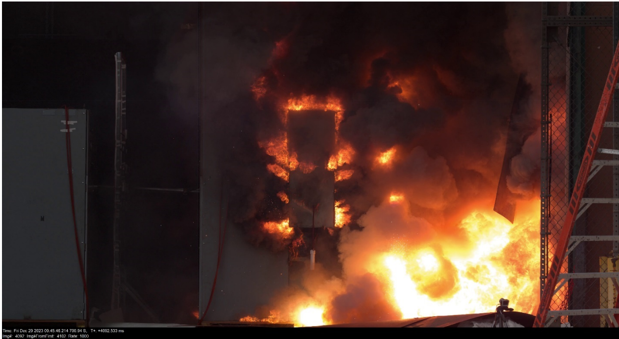
Figure 3-32: Test 2-38 imaged through 4k camera – camera imaging at 1000 fps – 4 seconds into the test. A fireball is now engulfing the east side of the test bay.
