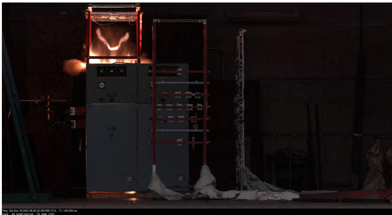
Figure 3-40: Test 2-39 imaged through 4k camera first millisecond into the test – camera imaging at 1000 fps – showing a v-shape object being ejected on the top, similar to Test 2-37 where the front access door was also ejected.
