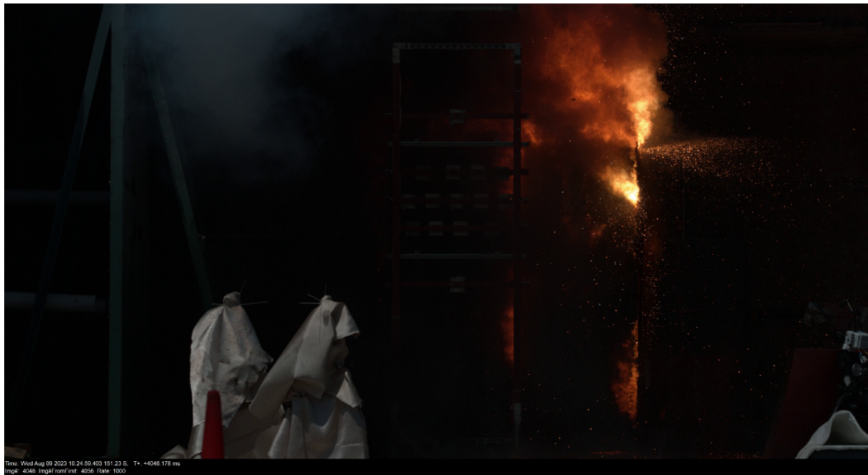
Figure 3-4: Test 2-35 imaged through 4k camera – notice fireball venting from adjacent enclosure and burning particulate ejection – camera imaging at 1000 fps.
