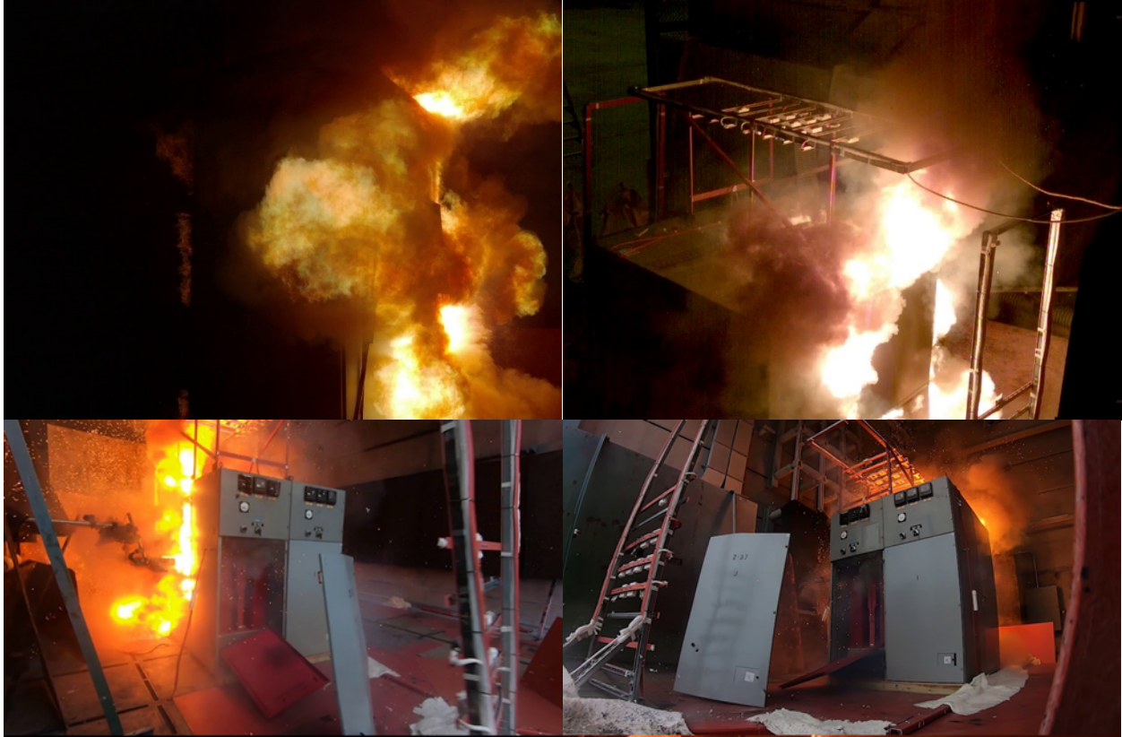
Figure 3-15: From top left (clockwise): v1310 while there is venting in the adjacent enclosure; v7 elevated from the northeast of the test while the west side enclosure vents in the back; GoPro outside southwest while access door is being ejected; GoPro outside floor southeast view of the same event. Notice instrument stand is being pushed by the ejected door.
