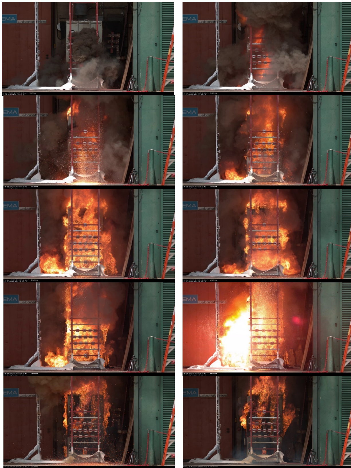
Figure 4-11: Test 2-33B imaged through 4k camera. Test that lasted 8 seconds. Pictures are shown at ~1 second intervals during the test (sequenced left to right, top to bottom) – camera imaging at 500 fps.
