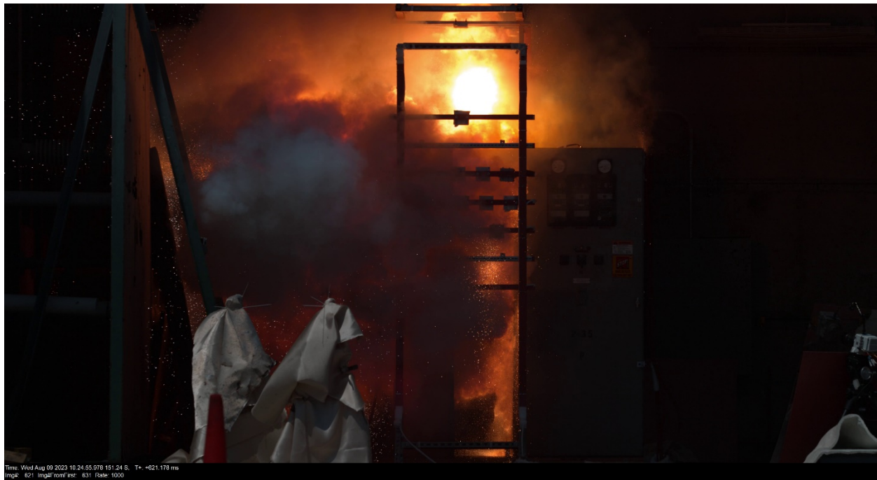
Figure 3-3: Test 2-35 imaged through 4k camera – notice enclosure door blown open and venting on top – camera imaging at 1000 fps.
