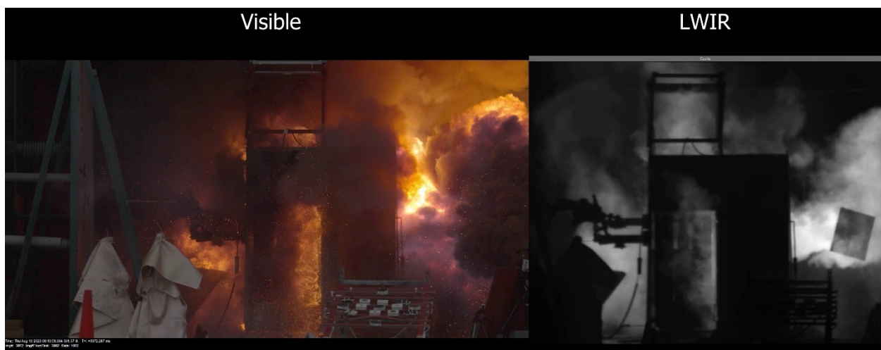
Figure 3-18: Sample frames from synchronized video of 4k and LWIR cameras close to 4 seconds into the test. Notice that the IR shows panel being ejected on the right side.
