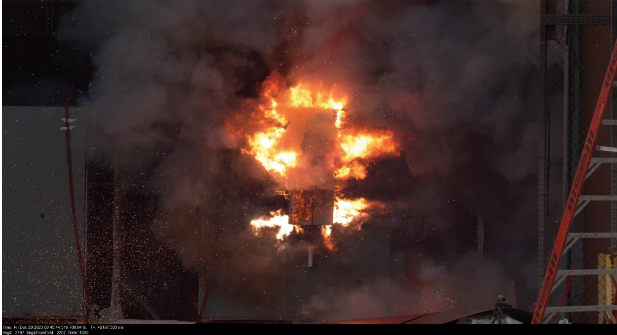
Figure 3-31: Test 2-38 imaged through 4k camera – camera imaging at 1000 fps – 2 seconds into the test. Burning metal particles are flying out from both adjacent enclosures and the south enclosure is venting fire through its southern panel. Notice the smoke engulfing the test bay.
