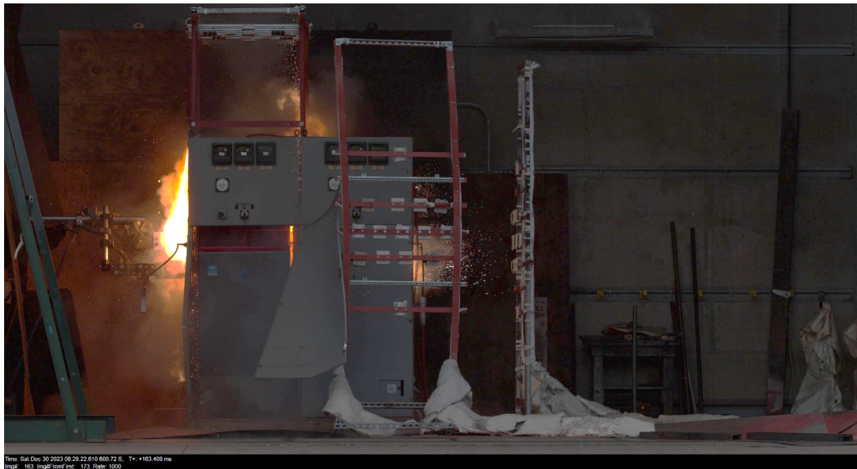
Figure 3-42: Test 2-39 imaged through 4k camera 120 ms after the previous image in Figure 3-40 – camera imaging at 1000 fps – showing access door hitting the instrument stand.
