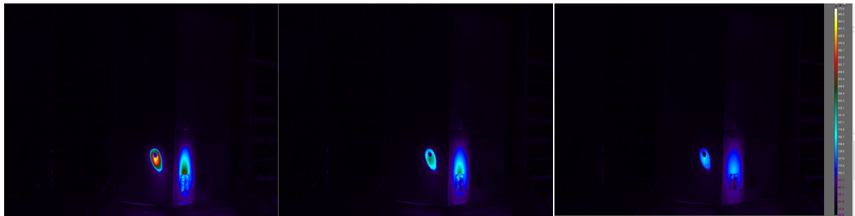
Figure 4-9: Temperature images from the LWIR camera A655 through 1 minute intervals, starting ~1 minute after the test. Arc is induced in the west most enclosure (red hot on top). Temperature ranges from 28.9 to 375 °C.
