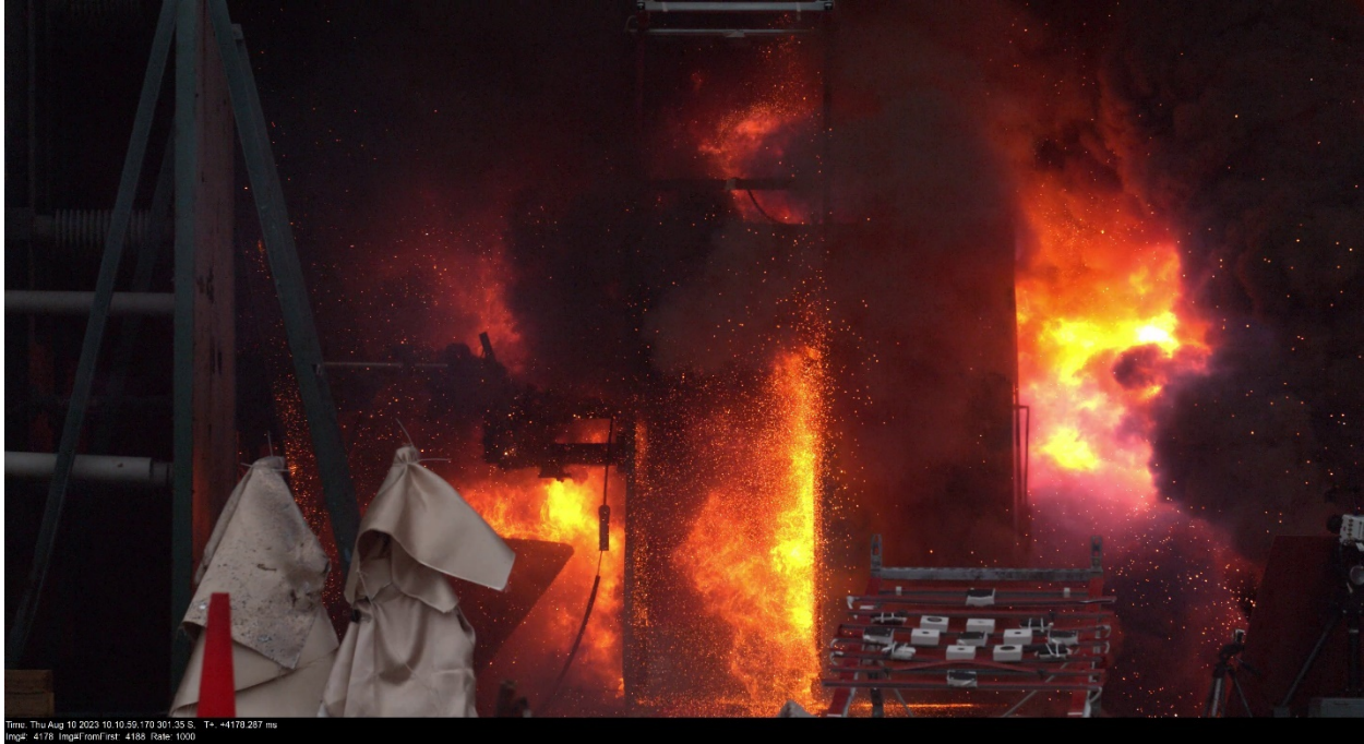
Figure 3-14: Test 2-37 imaged through 4k camera 3.5 seconds into the test – camera imaging at 1000 fps – The second enclosure ejecting a large fireball in side pointing north (this has been going on for half a second), while the first enclosure is consumed by the fire and ejecting sprays of burning metal particulate to the south.
