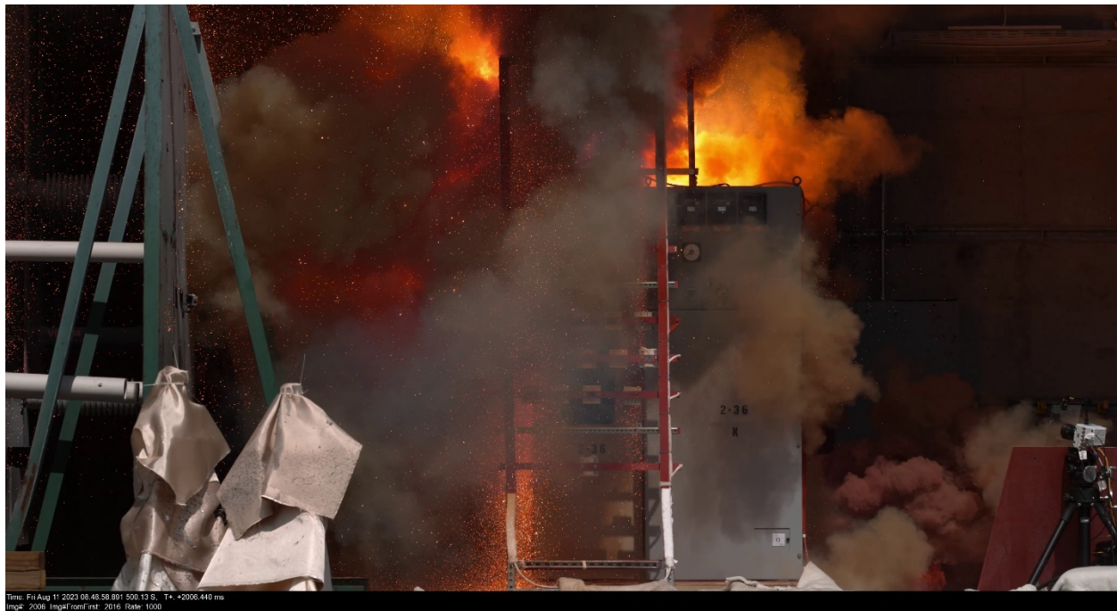
Figure 3-22: Test 2-36 imaged through 4k camera – camera imaging at 1000 fps – 2 seconds into the test. The view from the south seems to be dominated by dark smoke and there is fire activity in the north side.
