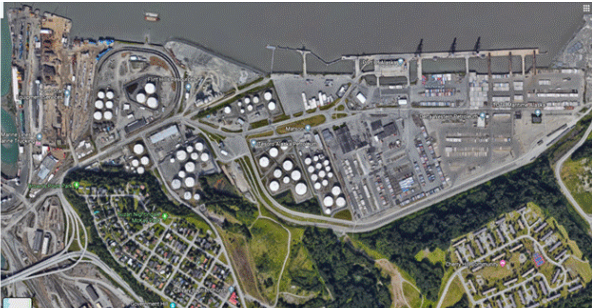
Figure 20. Aerial view of Port of Alaska. A dock with three gantry cranes, fuel storage and handling infrastructure, and container stacking areas are visible.
