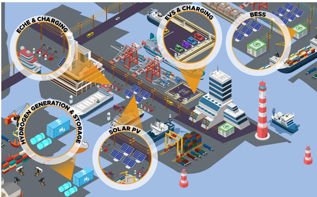
Figure 7. Examples of potential electrification-related deployments at a port, including LD EV charging, ECHE charging, solar PV, vessel shore power, and a BESS.
